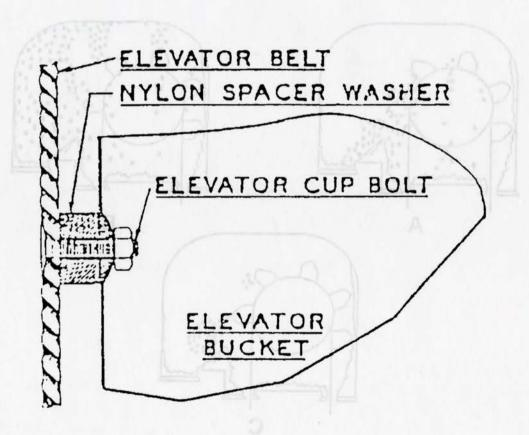
Figure 2. Spacer washer placed between belt and bucket to prevent mixtures. Recommend washer size: 1 in. dia. and 05 in. thick. apout to an adjacent outlet where seeds continue down that spout and into another bin or conveyor and varietal mixing occurs.
