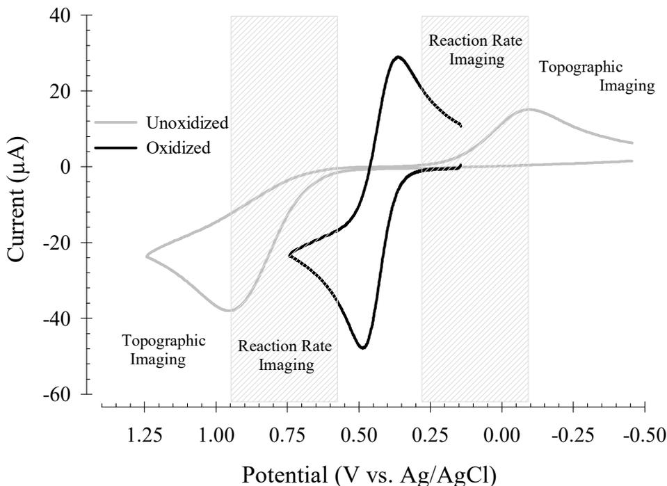
Fig. 1. Background subtracted cyclic voltammetry for a 3 mm GCE in a cell containing 2 mM  $\text{Fe}(\text{ClO}_4)_2$  in 1 M  $\text{H}_2\text{SO}_4$  before and after an intentional electrochemical oxidation of the electrode surface. 100 mV/s scan rate. The shaded regions indicate regions of applied substrate potentials suitable for use in reaction-rate imaging mode. The oxidation procedure is described in the text.
