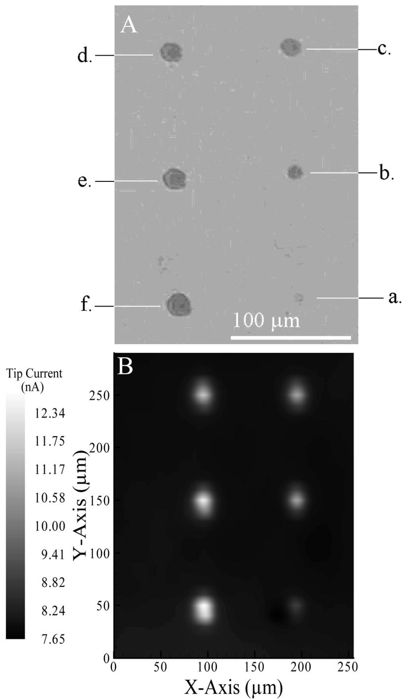
Fig. 7. Photomicrograph (A) and SECM reaction-rate image (B) of a series of oxidized spots formed by direct-mode oxidation using the following current densities at each labeled spot: (a) 0.014, (b) 0.07, (c) 0.14, (d) 0.21, (e) 0.28, and (f) 0.35 A/cm<sup>2</sup>.
