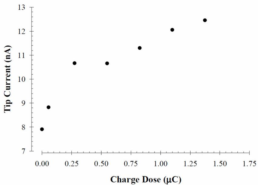
Fig. 8. Plot of measured tip current over each spot in the SECM image shown in fig. 7 versus the total charge “injected” in the oxidation step performed at each spot.
