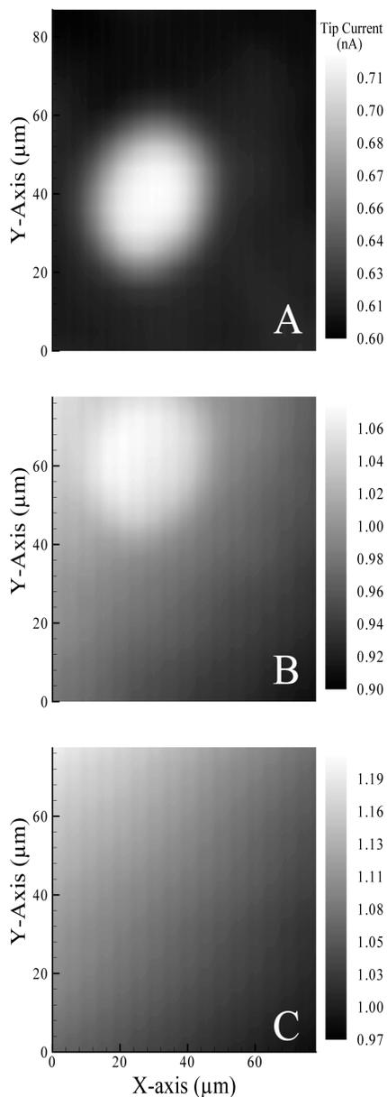
Fig. 4. SECM reaction-rate mode images of a spot of oxidized glassy carbon formed with the micro-reagent mode using  $\text{Ag}^{2+}$ . The conditions for the oxidation step are described in the text. The tip electrode was biased at 0.00 V while the substrate potentials for each image were (A) 0.80, (B) 1.00, and (C) 1.20 V vs. Ag/AgCl.
