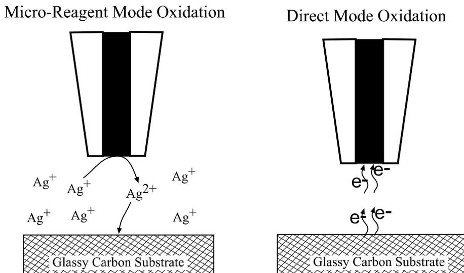
Fig. 3. Illustration of the two modes used for localized oxidation of the carbon surface by the SECM tip.
