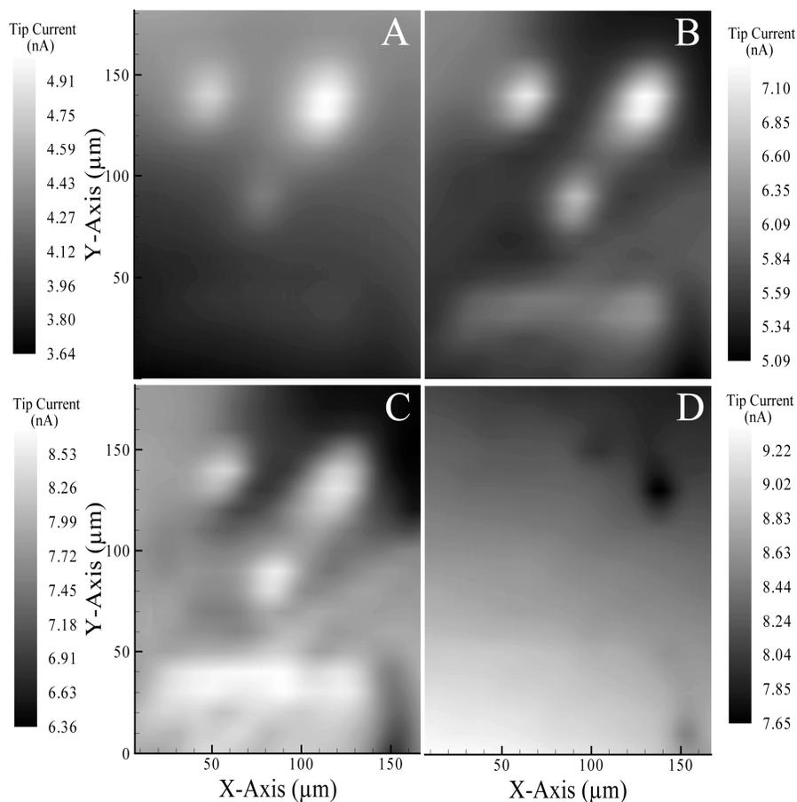
Fig. 6. SECM reaction-rate mode images of a pattern of oxidized spots and a line formed with the direct mode oxidation using a 10  $\mu\text{m}$ -dia. tip. The oxidation procedure is described in the text. The tip electrode was biased at 0.80 V while the substrate potentials for each image were (A) 0.243, (B) 0.043, (C) -0.243, and (D) -0.443 V vs. Ag/AgCl.
