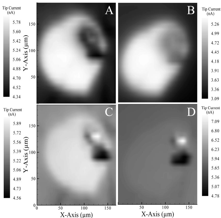
Fig. 5. SECM reaction-rate mode images of a region of oxidized carbon formed by the direct mode oxidation with a 100- $\mu\text{m}$  dia. tip. The tip electrode was biased at 0.80 V while the substrate potentials for each image were (A) 0.243, (B) 0.043, (C) -0.243, and (D) -0.443 V vs. Ag/AgCl.
