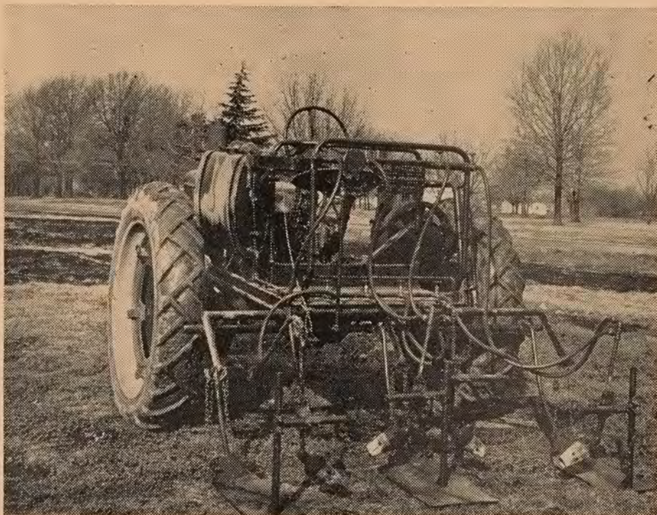
Figure 7. The flame cultivator. Picture furnished by Delta Branch Experiment Station.
