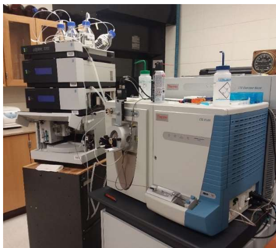
Figure 8: Nano-electro spray ionization LTQ-Orbitrap Velos mass spectrometer with an upstream Ultimate 3000 HPLC system, both from Thermo Fisher Scientific.
