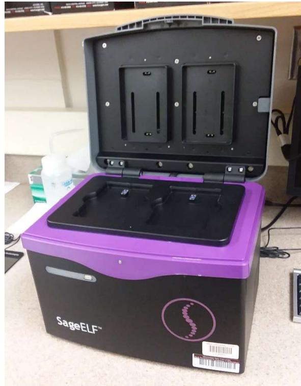
Figure 5: Sage Science SageELF electrophoretic system for whole sample fractionation of DNA or protein.
