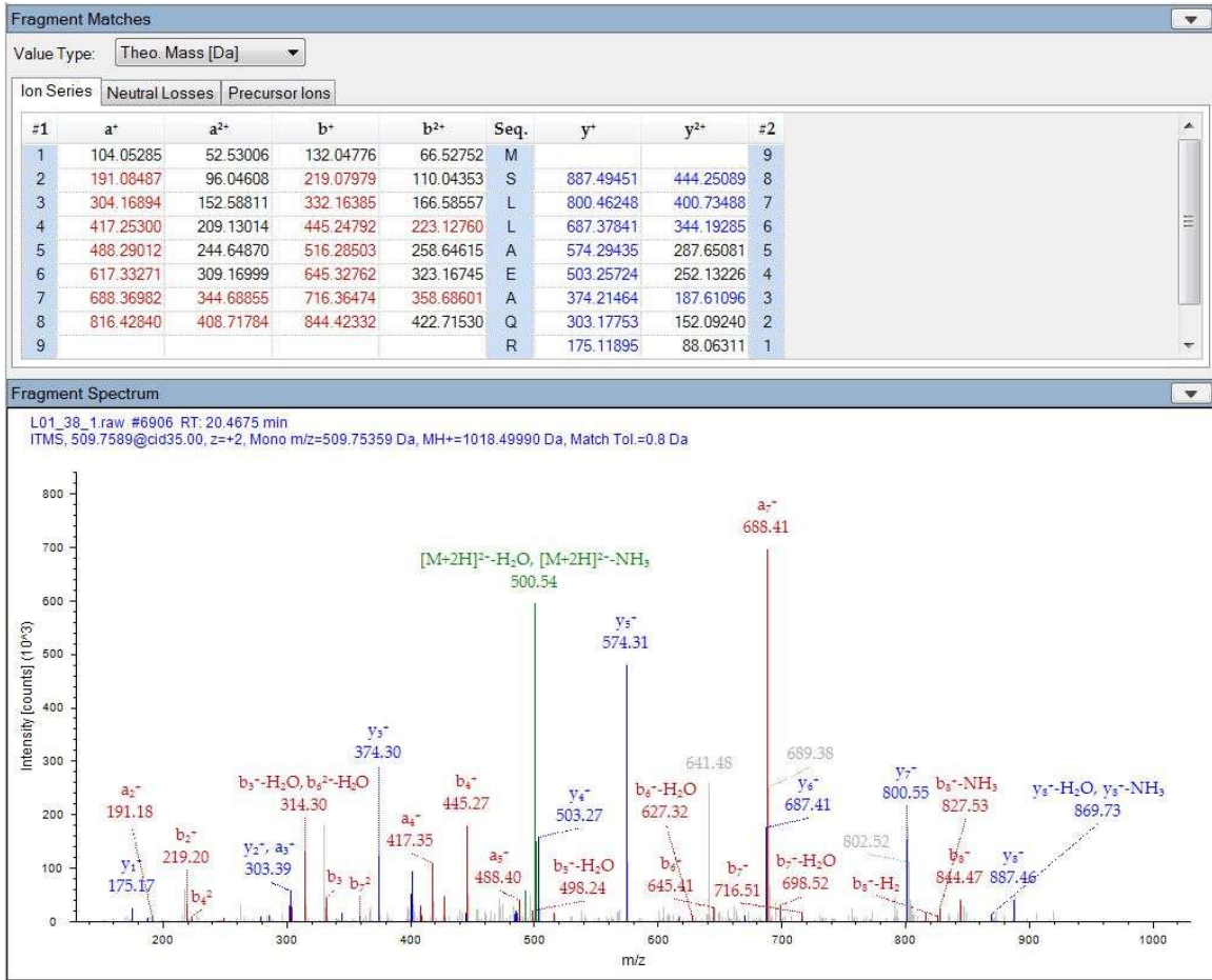
Figure 11: Identification of MSLLAEAQR peptide in fractionated sample of G. mustelinum leaf. Color-highlighted peaks in experimental MSMS spectra, and m/z values of respective ions were matched to theoretical data using Proteome Discover (Thermo) software and G. mustelinum protein database.
