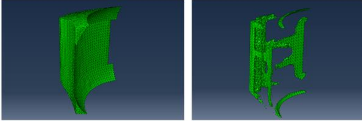
Figure 2.7 (a) Original part, (b) mass-optimized part after topology optimization
