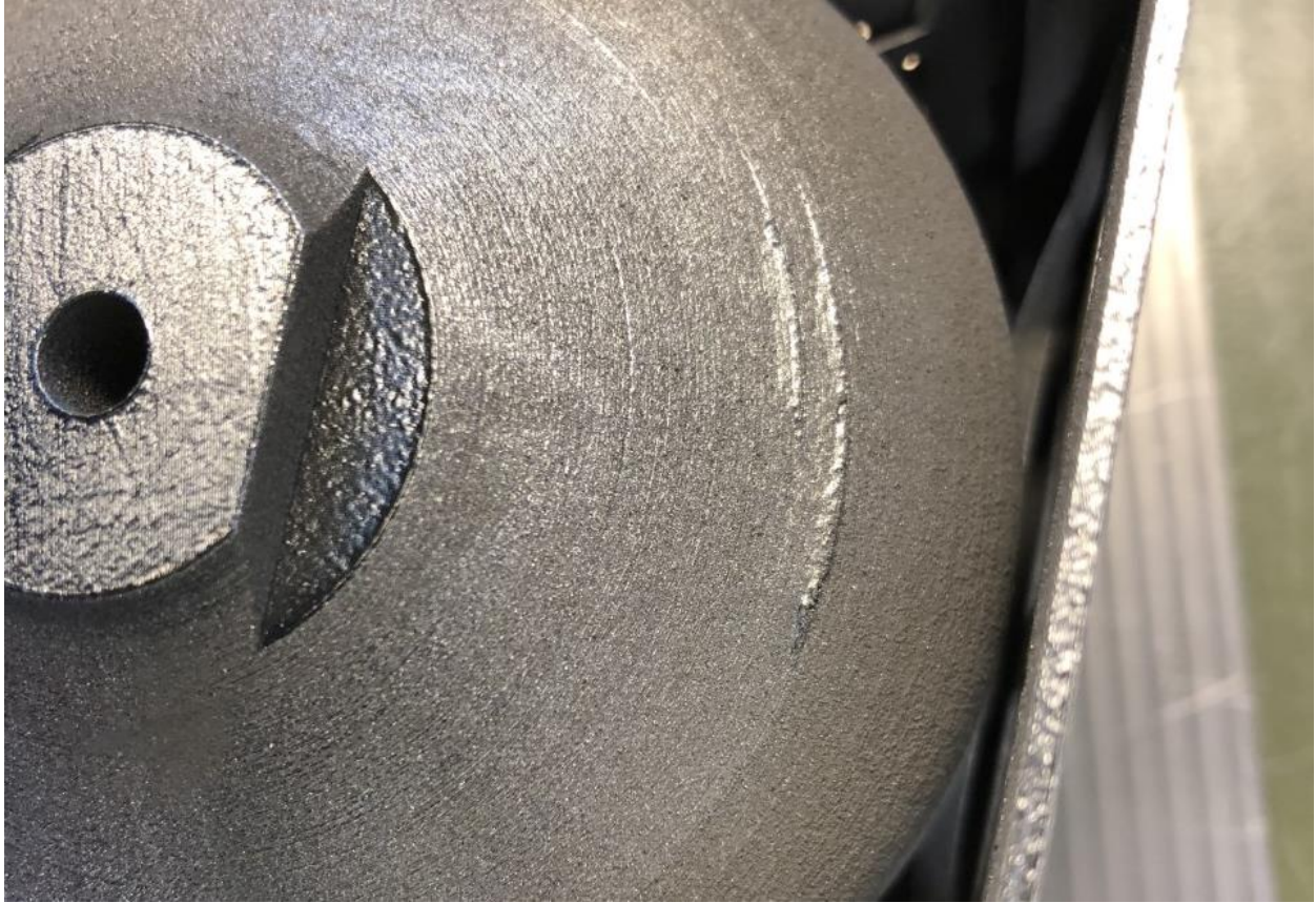
Figure 3.16 Minor absence of adhesion on upper pressure vessel
