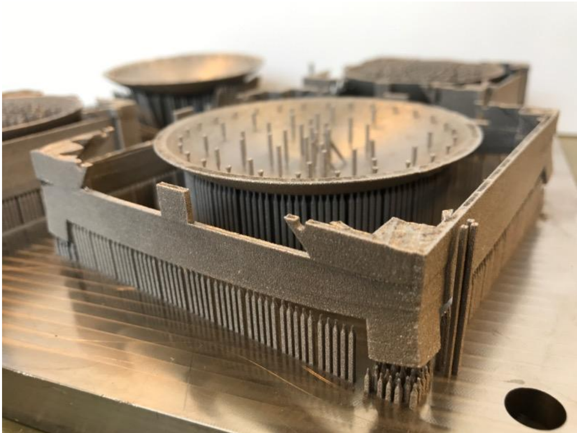
Figure 3.11 Example of bowing defect in the CubeSat
