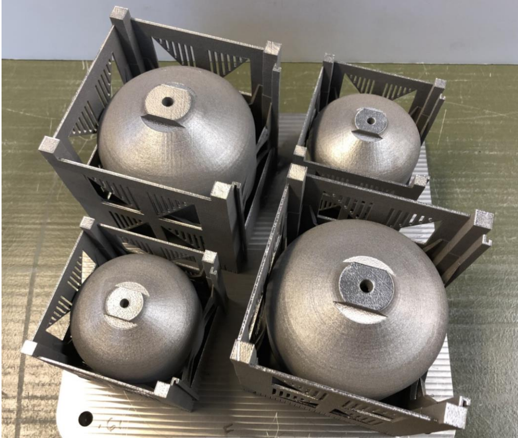
Figure 3.14 Top view of completed CubeSat build
