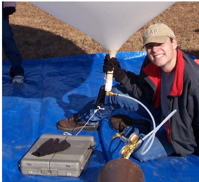
Figure 3.8 Balloon Inflation Configuration
