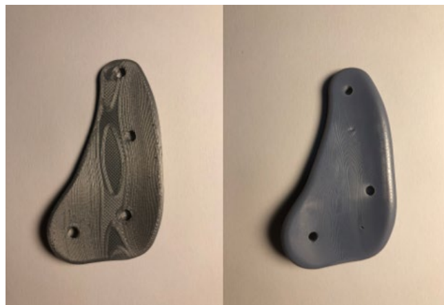
Figure 1.1 Surface Quality of FDM and SLA Printers
