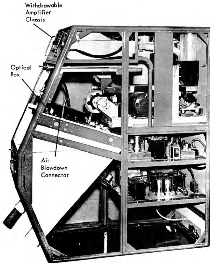
Figure 1. Side View of a Sortex G. 414 Machine
