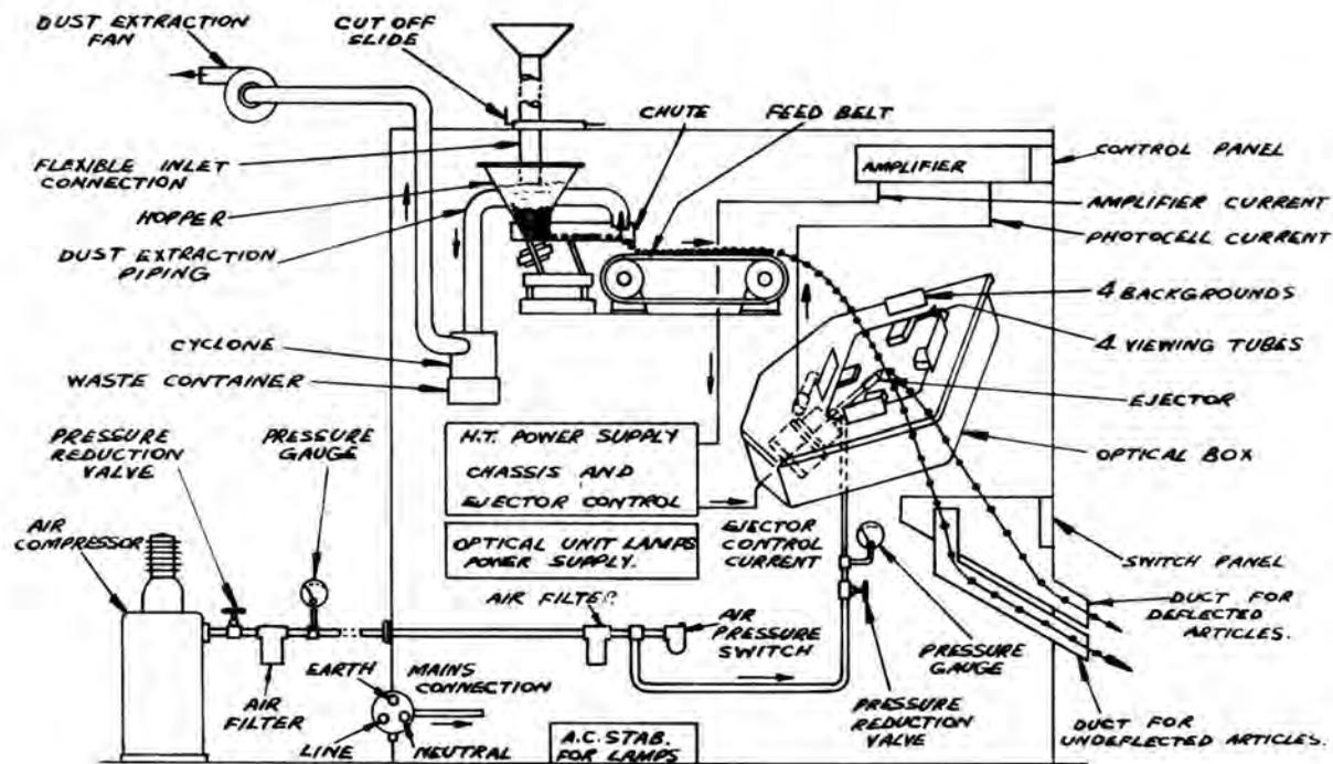
Figure 2. Schematic diagram of the mechanical system for the Sortex G. 414 and G. 415 machines
