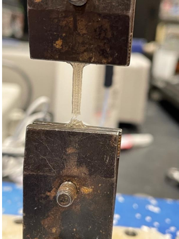
Figure 5.2 PLGA-KGN specimen rupture during tensile testing
