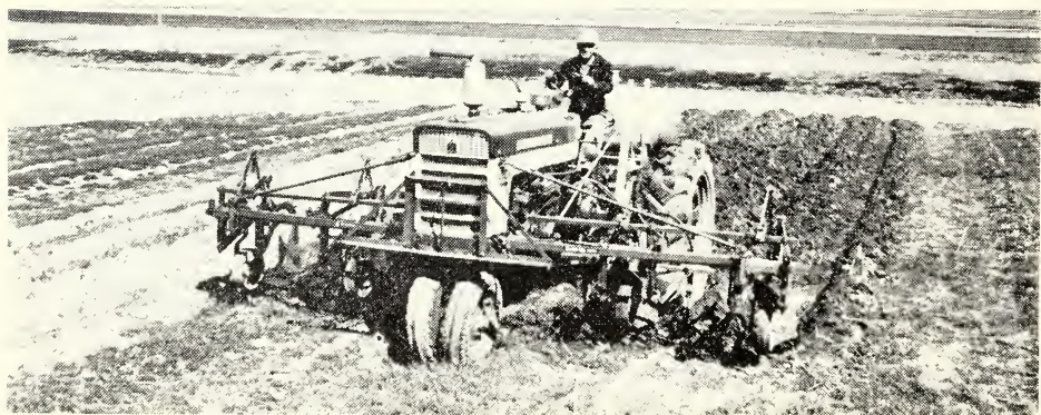
Figure 2. This tractor is equipped for applying anhydrous ammonia and preparing four uniform seedbeds in 1 operation.
