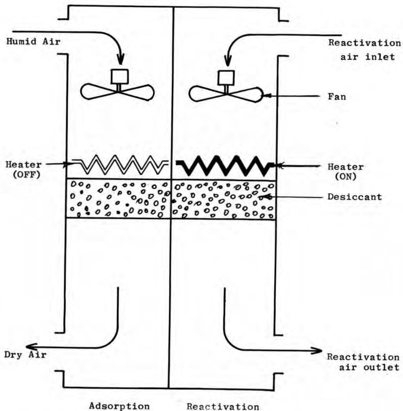
Figure 3. Schematic diagram of an adsorption dehumidifier.
