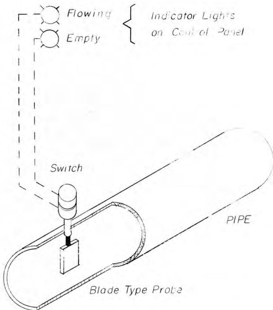
Drawing No. 4 shows a unit similar to the previous one for conveyor status determination. The same unit is used, however, it is installed in a system where the seed are being pneumatically conveyed.
