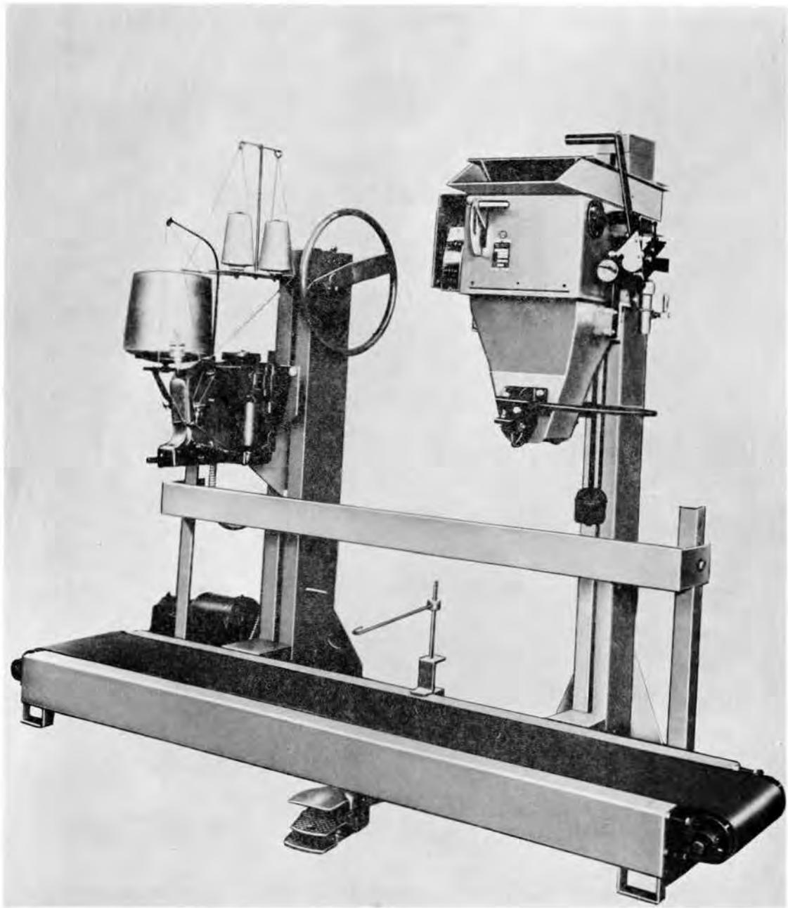
Figure 1. Equipment for a one-man bagging operation.
