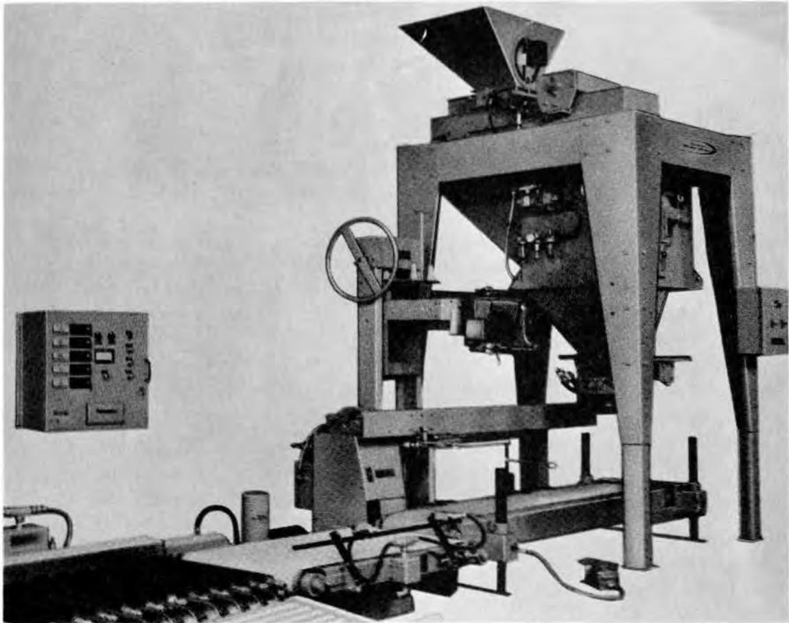
Figure 2. A typical installation of an automatic packaging system.
