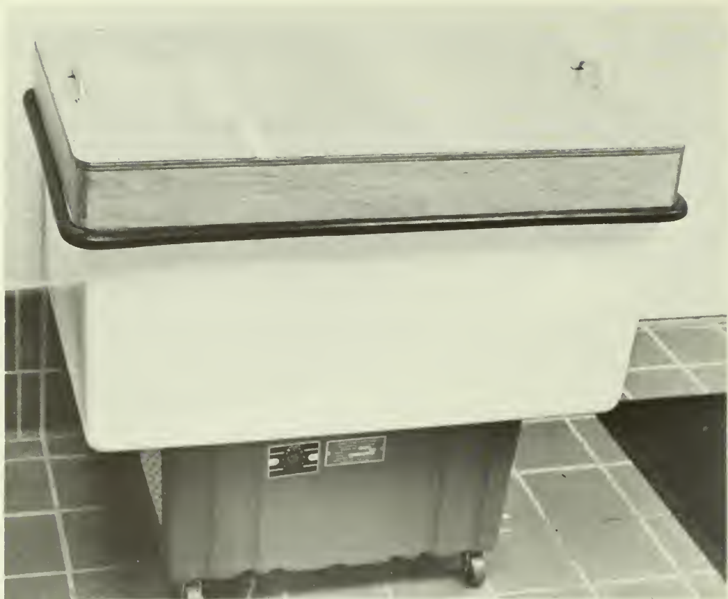
Fig. 2. Freezing unit with insulated cover closed.
