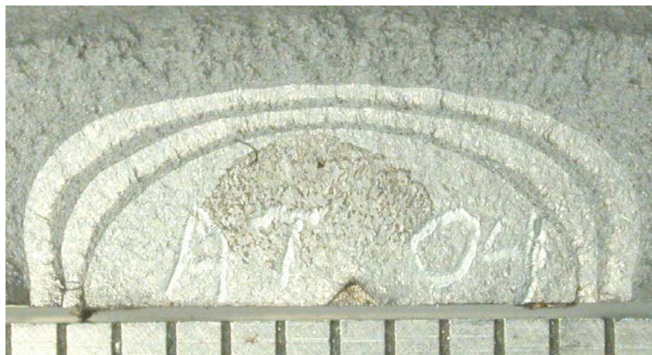
Figure 3-2.a Typical Surface Crack Fracture Surface (Tension)
