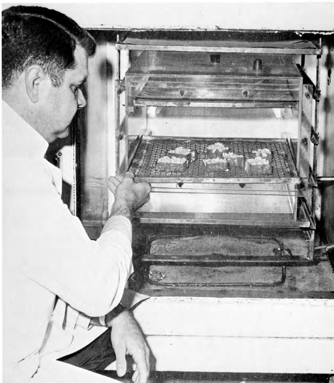
Figure 1. Interior view of an accelerated aging chamber.
