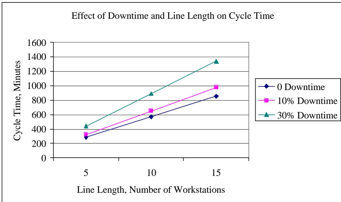
Figure 26. Effect of Downtime and Line Length on Cycle Time
