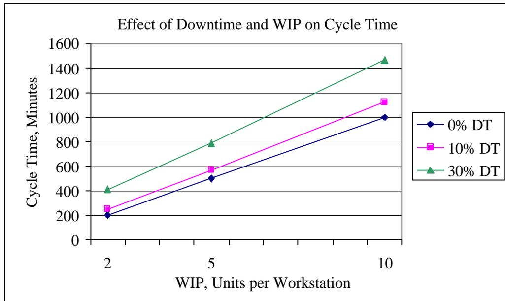
Figure 22. Effect of Downtime and WIP on Cycle Time
