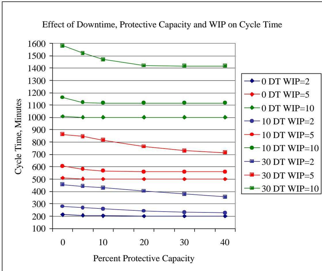
Figure 14. Effect of Downtime, PC, and WIP on Cycle Time
