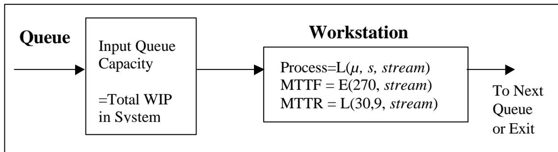
Figure 1. Processing and Downtime Distributions Set-up for Each Workstation
