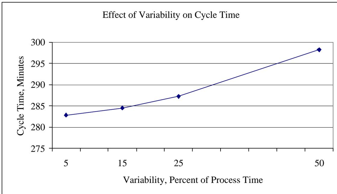
Figure 7. Effect of Variability on Cycle Time
