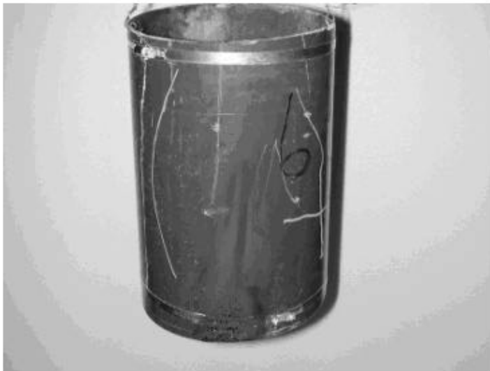
The Tracking Appeared on the External Surface of the Sample (No.6, With Same Scratches) After a 5 Hour Aging in Salt Fog Plus 25 kV/ft Electrical Stress.
