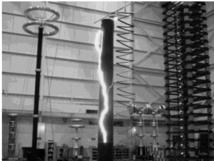
The CFO Voltages of 35 kV Porcelain Pin Insulators Plus Fiberglass Poles Were Evaluated under Dry Conditions. The Tested Pole Length Is 8 Feet. The Discharge Path Consists of the Insulator Surface and the External Surface of the Pole.
