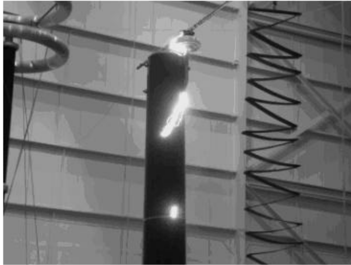
The CFO Voltages of 35 kV Porcelain Pin Insulators Plus Fiberglass Poles Were Evaluated under Dry Conditions. The Tested Pole Length Is 3 Feet. The Discharge Path Consists of the Insulator Surface and Both Sides of Pole's Surfaces.
