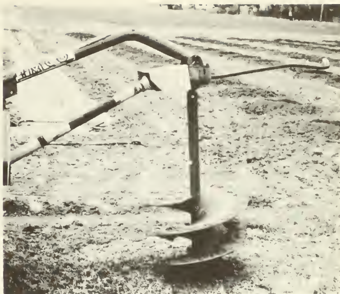
Figure 2. Blueberry planting sites can be prepared using a middle-buster (left) to open rows or by digging a hole with a tractor mounted auger (right).
