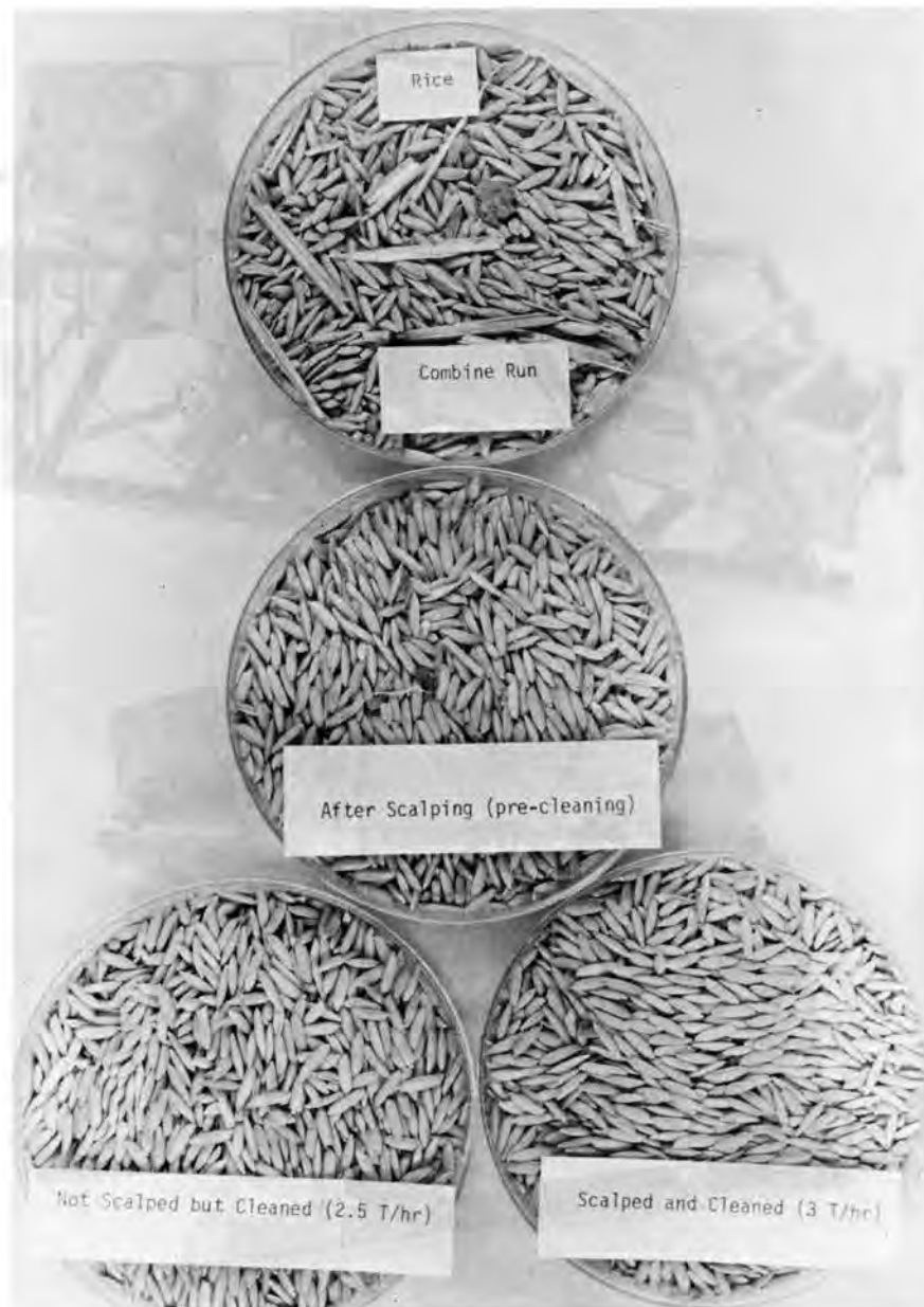
Figure 1. Combine-run rice seed (above) the same seed after scalping (middle). Rice seed after cleaning with an air-screen cleaner (below). Note the influence of scalping on the cleaning capacity.
