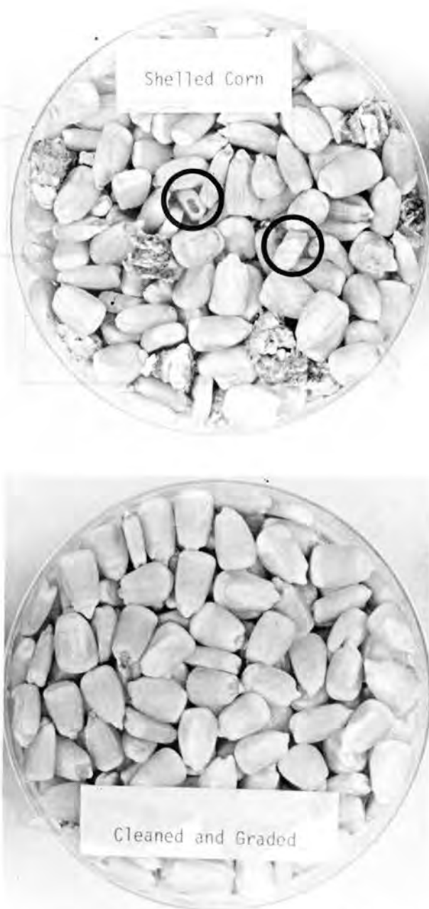
Figure 4. Seed corn as discharged from the sheller (above) note mechanical injury to kernels circled. Cleaned, size graded seed corn (below).
