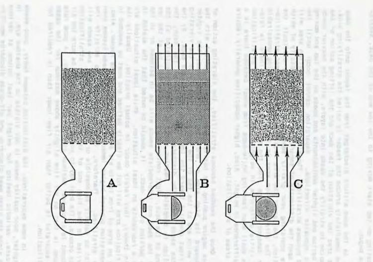
Figure 1. Gravity Table. (A) Fan intake closed; no stratification. (B) Proper volume of air flow through the deck; the seed layer is stratified. (C) Excessive volume of air flowing through the deck breaking the stratification.
