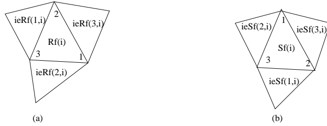
Figure 2.6: (a) Faces on the rotating surface and, (b) faces on the stationary surface face vertex indices and the corresponding convention for face neighbor data.
