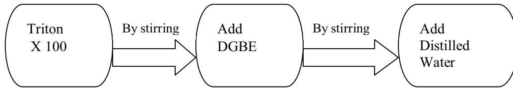
Fig. 2.3. Process of preparing skin mimicking material.
