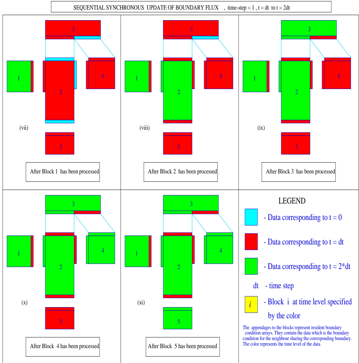
Figure 3.2: Synchronous update of boundary flux during the second time-step in the sequential algorithm
