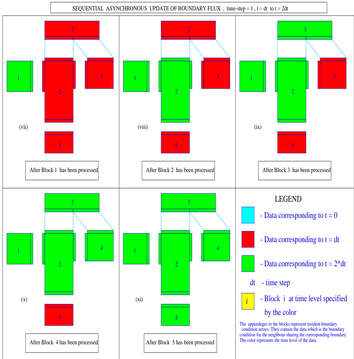
Figure 3.4: Asynchronous update of boundary flux during the second time-step in the sequential algorithm
