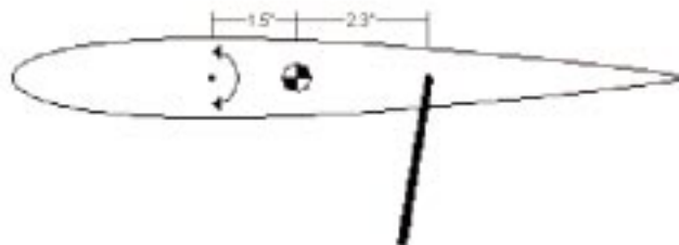
Figure 34. Blade Measurements Used in Bosch Cycloidal Propeller
