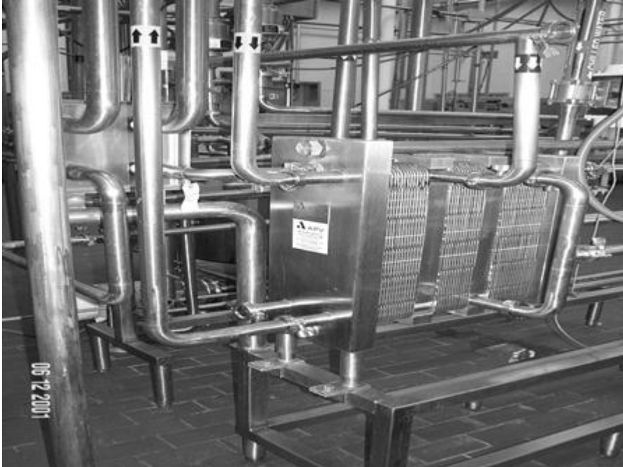
Figure 2 Plate pasteurizer, picture taken by Dr. William Gillis
