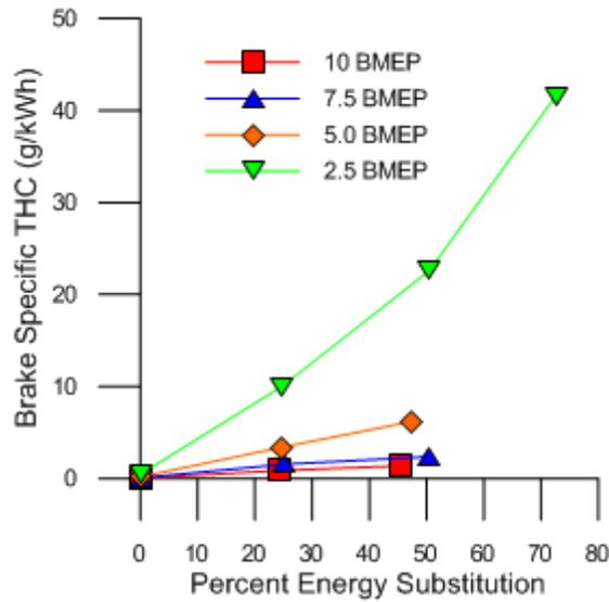
Figure 4.13 Brake specific THC emissions vs. PES for ULSD-propane dual fueling
