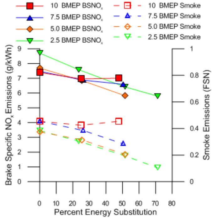
Figure 3.8 Brake specific NO<sub>x</sub> and smoke emissions vs. PES for B100-methane dual fueling
