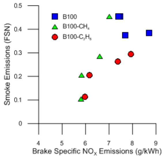
Figure 3.7 Smoke- $\text{NO}_x$  tradeoff for straight biodiesel and maximum PES of  $\text{C}_3\text{H}_8$  and  $\text{CH}_4$
