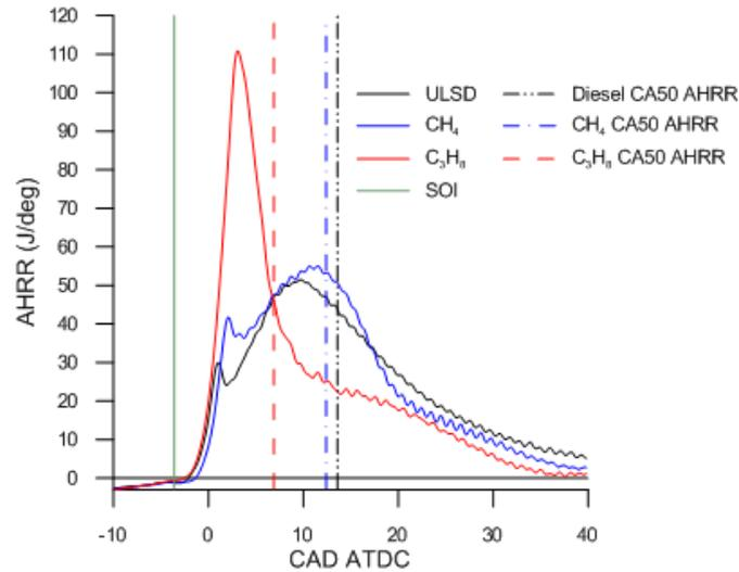
Figure 4.6 AHRR vs. CAD ATDC at 10 bar BMEP
