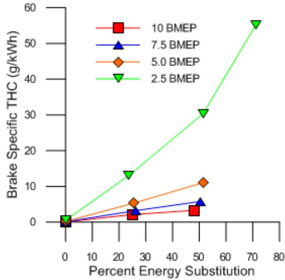
Figure 3.12 Brake specific THC emissions vs. PES for B100-methane dual fueling
