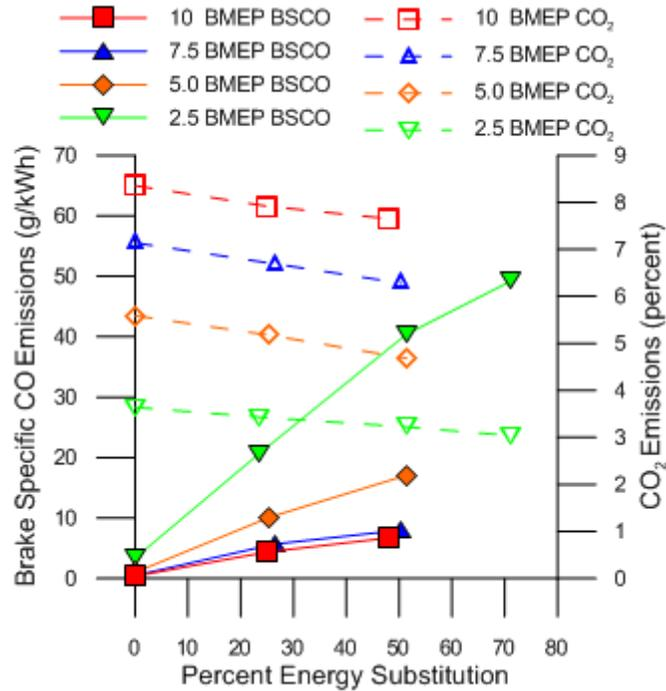
Figure 3.10 Brake specific CO and CO<sub>2</sub> emissions vs. PES for B100-methane dual fueling
