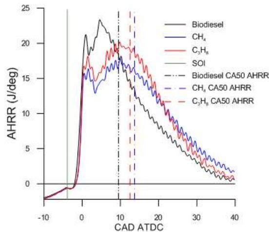
Figure 3.3 AHRR vs. CAD ATDC at 2.5 bar BMEP
