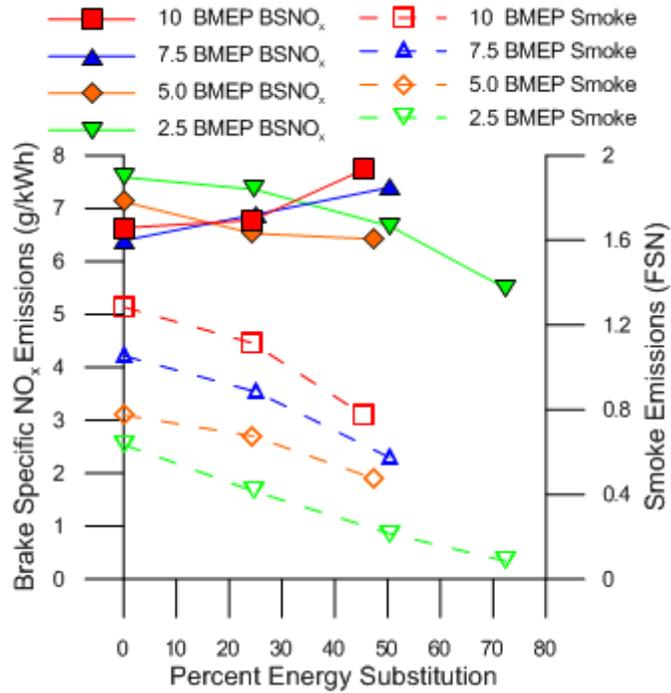
Figure 4.9 BSNO<sub>x</sub> and smoke emissions vs. PES for ULSD-propane dual fueling
