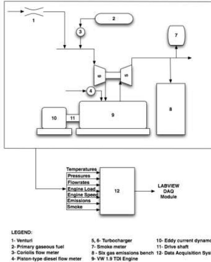
Figure 2.1 Schematic of the 1.9L VW experimental setup
