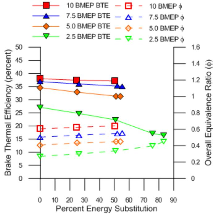
Figure 4.1 BTE and overall equivalence ratio vs. PES for ULSD-methane dual fueling
