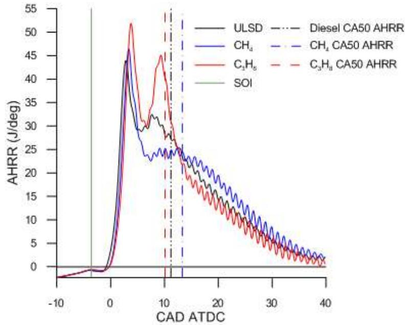
Figure 4.4 AHRR vs. CAD ATDC at 5 bar BMEP
