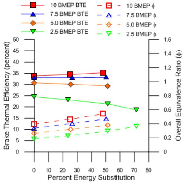
Figure 3.1 BTE and overall equivalence ratio vs. PES for B100-methane dual fueling
