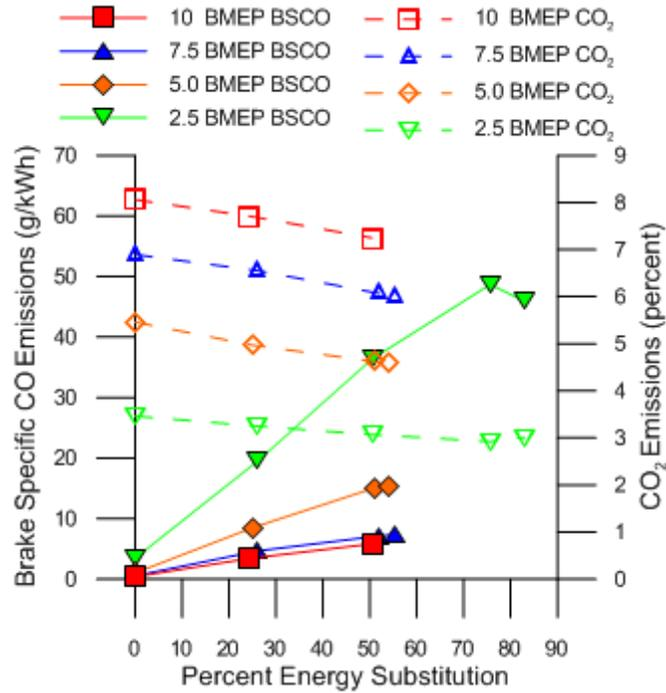
Figure 4.10 BSCO and CO<sub>2</sub> emissions vs. PES for ULSD-methane dual fueling
