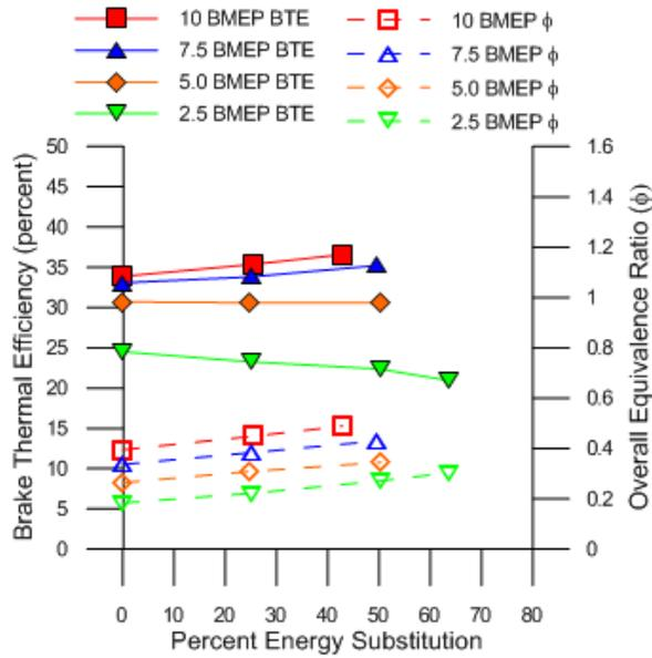
Figure 3.2 BTE and overall equivalence ratio vs. PES for B100-propane dual fueling
