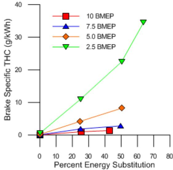
Figure 3.13 Brake specific THC emissions vs. PES for B100-propane dual fueling
