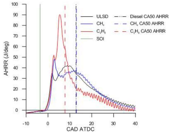
Figure 4.5 AHRR vs. CAD ATDC at 7.5 bar BMEP
