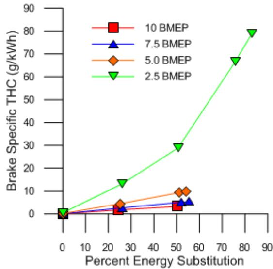
Figure 4.12 Brake specific THC emissions vs. PES for ULSD-methane dual fueling
