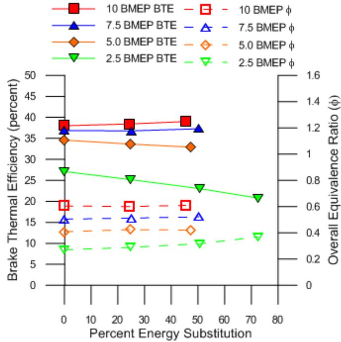
Figure 4.2 BTE and overall equivalence ratio vs. PES for ULSD-propane dual fueling
