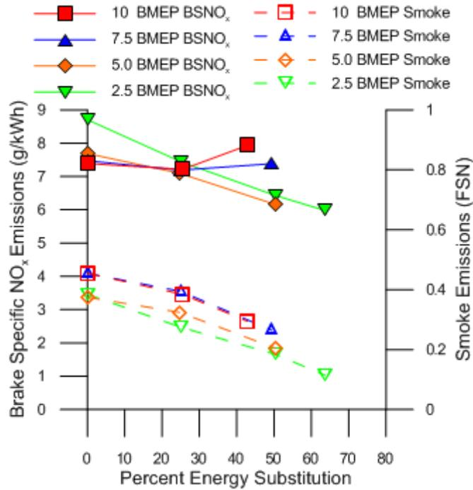
Figure 3.9 BSNO<sub>x</sub> and smoke emissions vs. PES for B100-propane dual fueling
