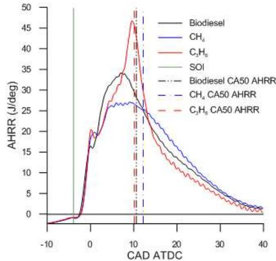
Figure 3.4 AHRR vs. CAD ATDC at 5 bar BMEP
