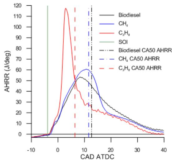
Figure 3.6 AHRR vs. CAD ATDC at 10 bar BMEP
