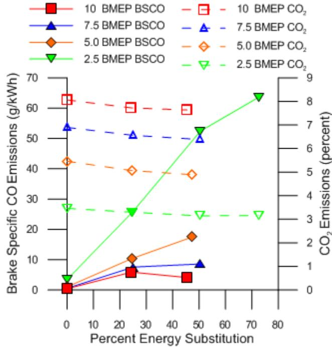
Figure 4.11 BSCO and CO<sub>2</sub> emissions vs. PES for ULSD-propane dual fueling
