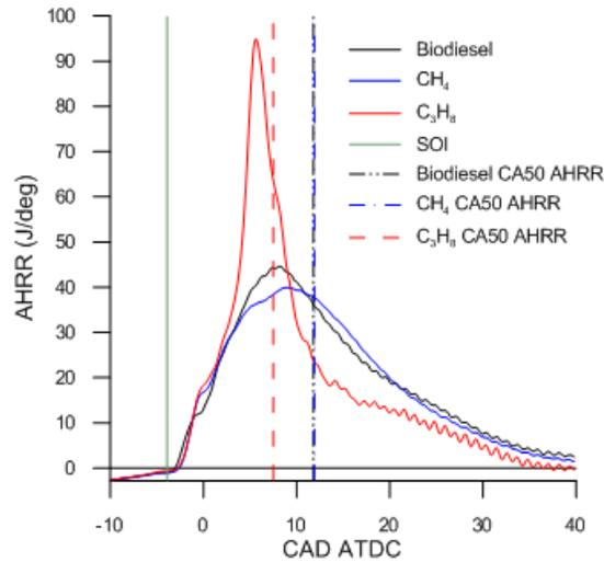
Figure 3.5 AHRR vs. CAD ATDC at 7.5 bar BMEP
