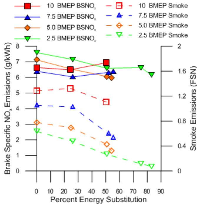
Figure 4.8 BSNO<sub>x</sub> and smoke emissions vs. PES for ULSD-methane dual fueling.
