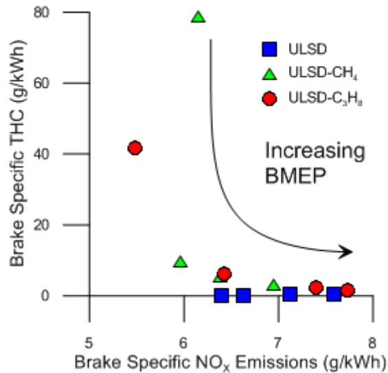
Figure 4.14 Brake specific THC emissions vs. BSNO<sub>x</sub> tradeoff at various loads and maximum PES for straight ULSD, ULSD-methane and ULSD-propane dual fueling
