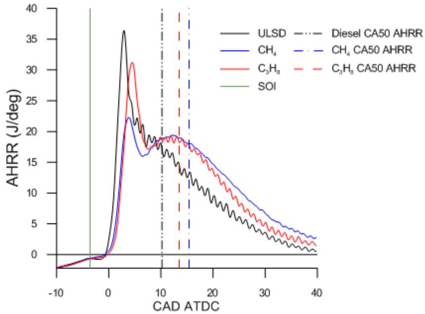
Figure 4.3 AHRR vs. CAD ATDC at 2.5 bar BMEP
