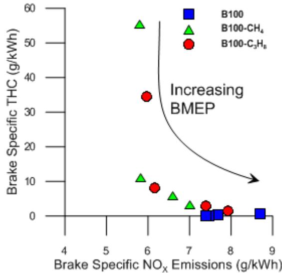
Figure 3.14 Brake specific THC emissions vs. BSNO<sub>x</sub> tradeoff at various loads and maximum PES for straight biodiesel, B100-methane and B100-propane dual fueling
