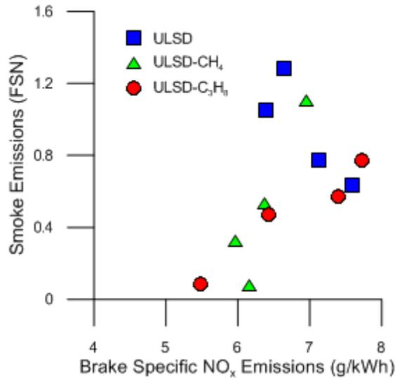
Figure 4.7 Smoke- $\text{NO}_x$  tradeoff for straight ULSD and maximum PES of  $\text{C}_3\text{H}_8$  and  $\text{CH}_4$
