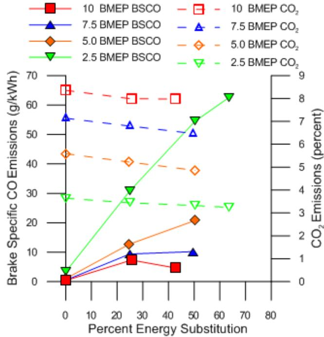
Figure 3.11 Brake specific CO and CO<sub>2</sub> emissions vs. PES for B100-propane dual fueling
