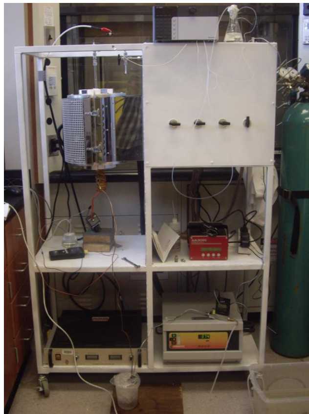
Figure 3.3 Electro-spray unit retrofitted to the reformer
