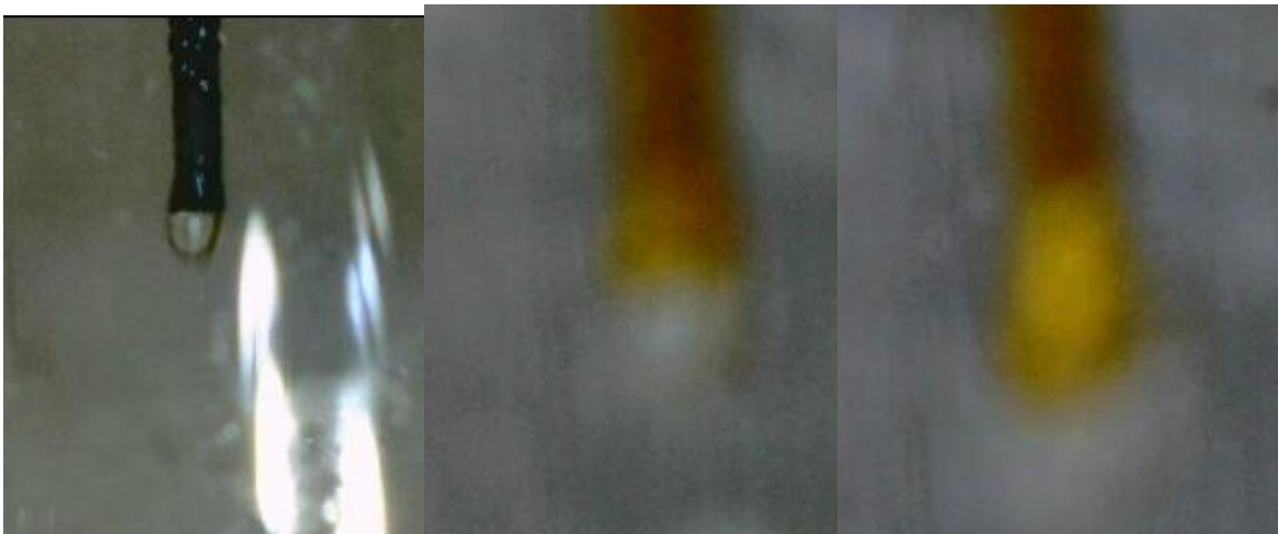
Figure 4.2 Cone jet spray formation of glycerol feed with high voltage
