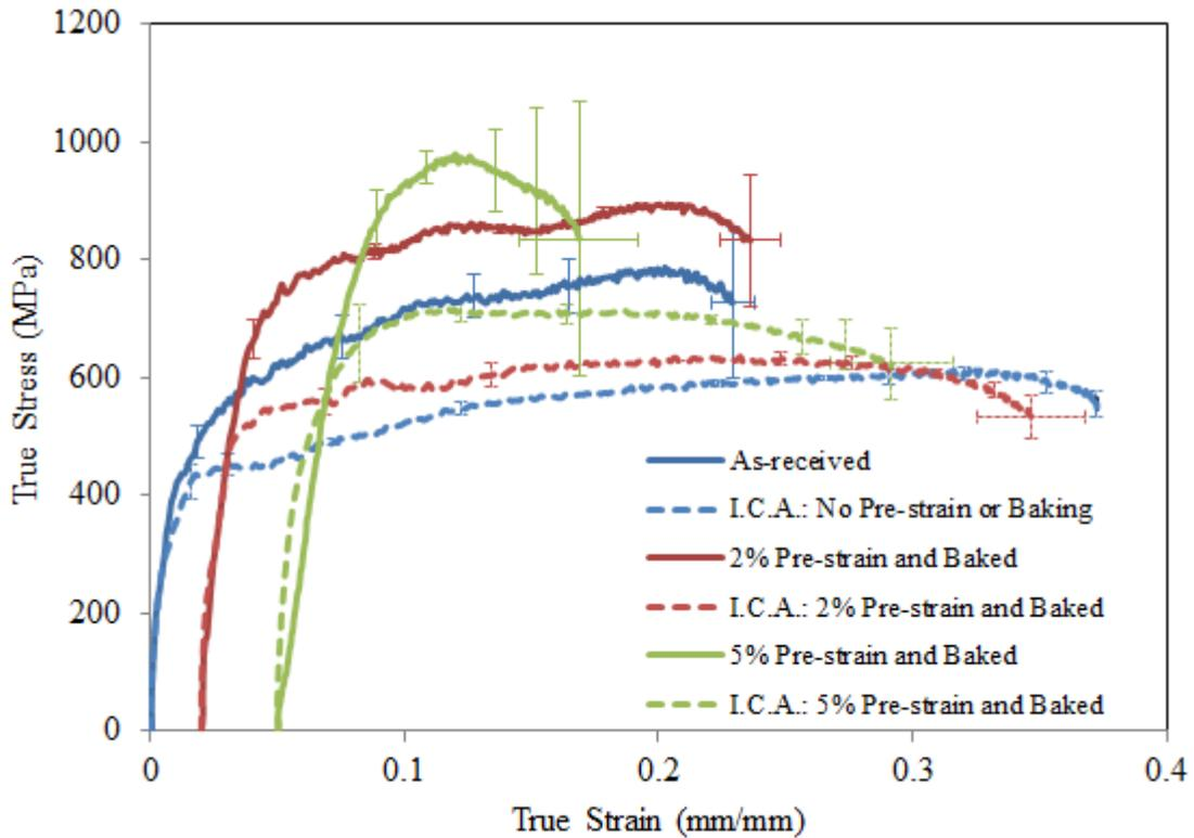
Figure 3.16 True stress vs. true strain graph resulting from high strain-rate tensile tests of the I.C.A. series.
