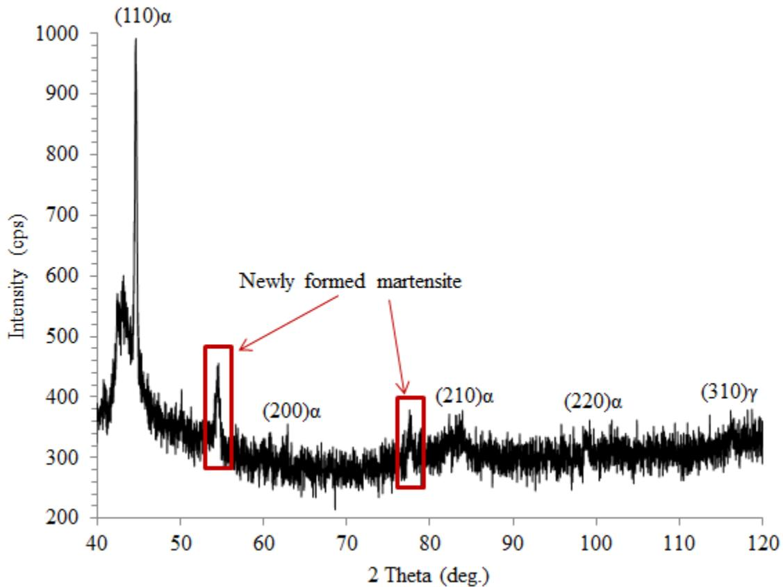
Figure 3.14 XRD Analysis of the TRIP steel series with the five major absorption peaks indexed.
