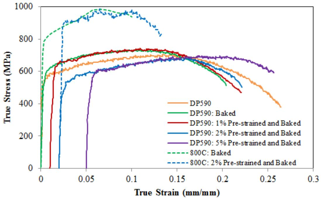
Figure 2.12 Stress versus strain curves resulting from high strain-rate tensile tests
