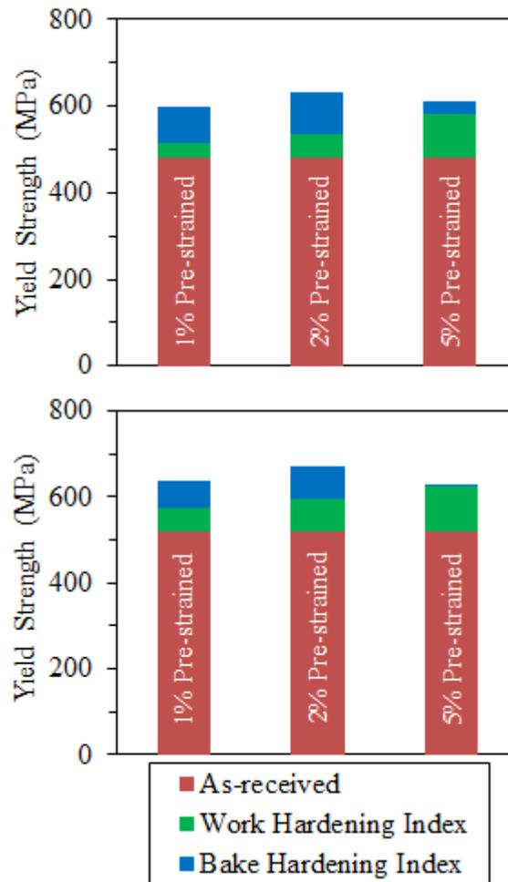
Figure 2.8 Work- and bake-hardening indices for their respective quasi-static tests.
