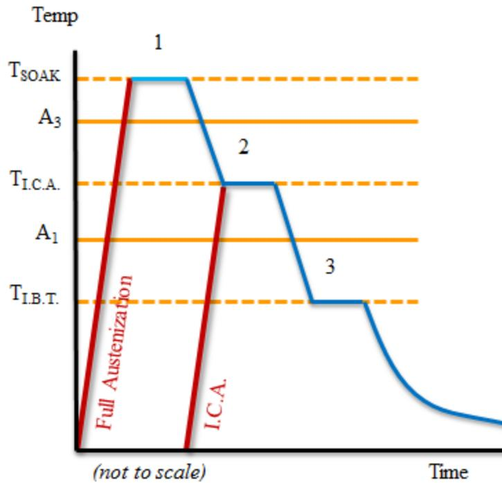
Figure 3.2 Heating/cooling schematic showing typical cooling schedules.
