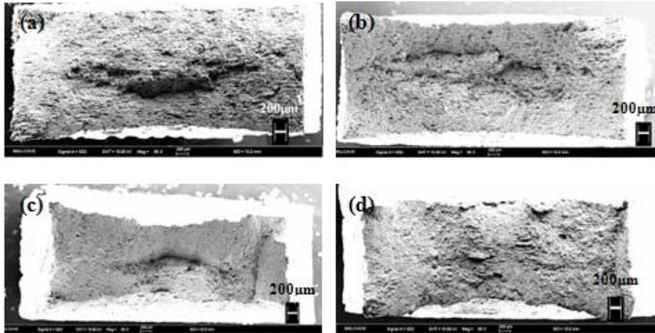
Figure 2.11 SEM fractography revealing fracture surfaces on the annealed series resulting from quasi-static testing.
