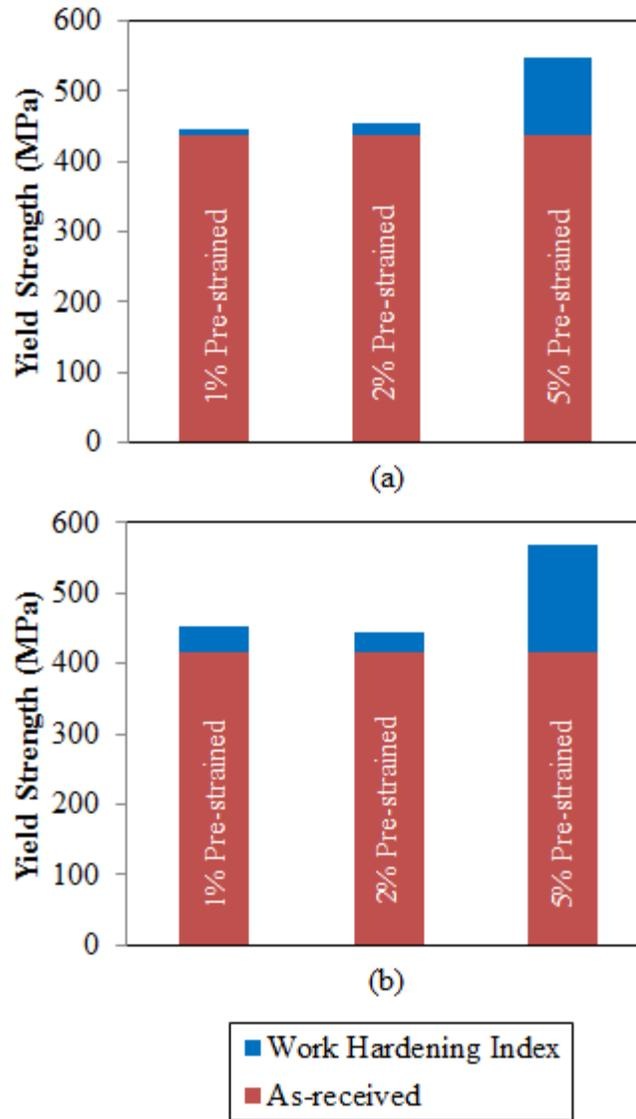
Figure 3.7 Work-hardening indices with respect to various thermo-mechanical preconditioning protocols.
