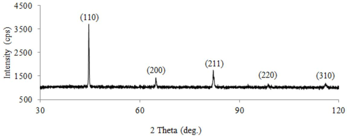
Figure 3.4 XRD scan from as-received TRIP680.
