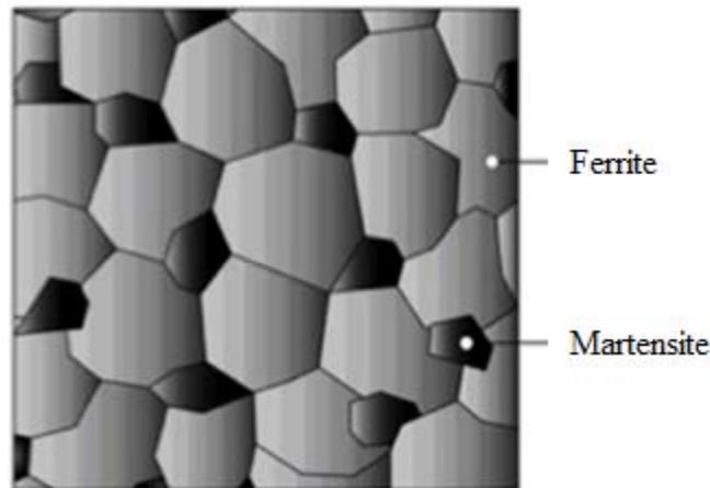
Figure 2.1 Schematic of DP steel showing the interspersed phases of ferrite and martensite.
