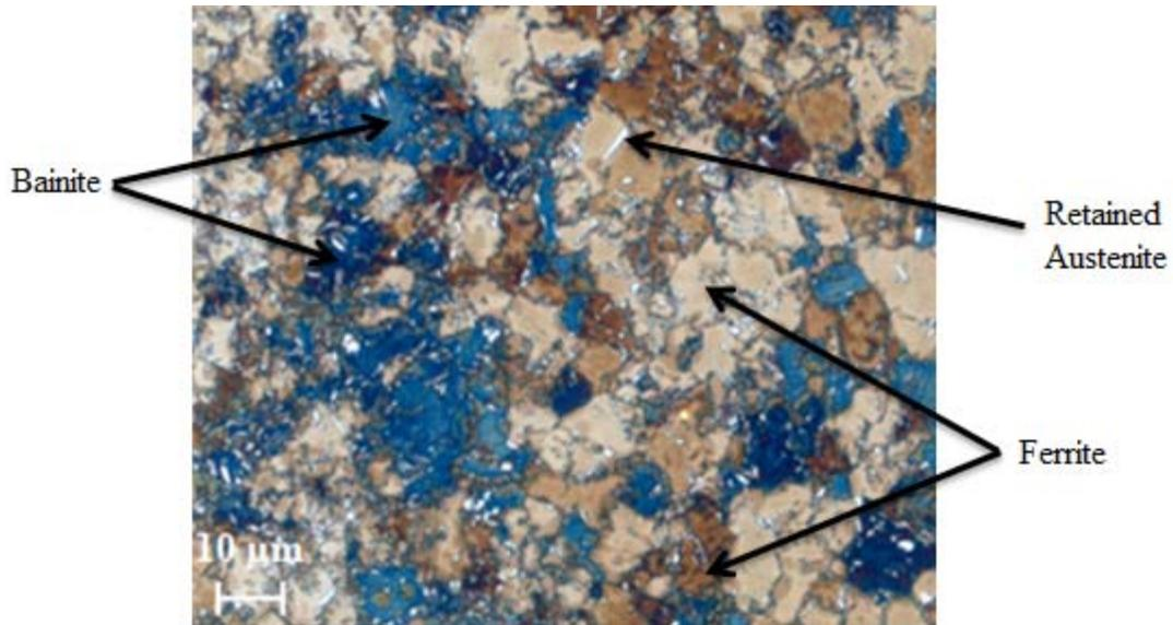
Figure 3.3 TRIP680 etched with Beraha's tint etchant: ferrite (tan and dark brown), bainite (blue), and retained austenite (bright white).
