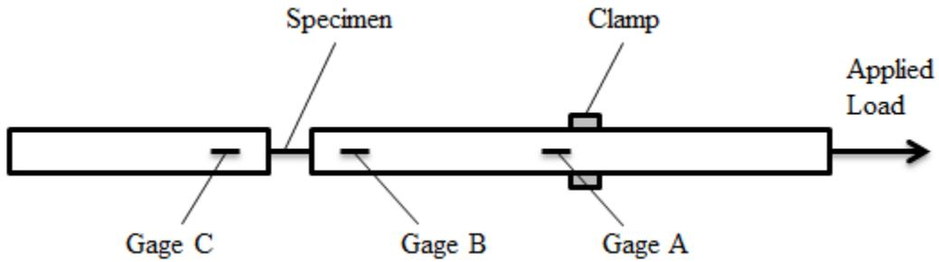
Figure 2.2 Schematic of tension SHB high strain-rate testing apparatus.
