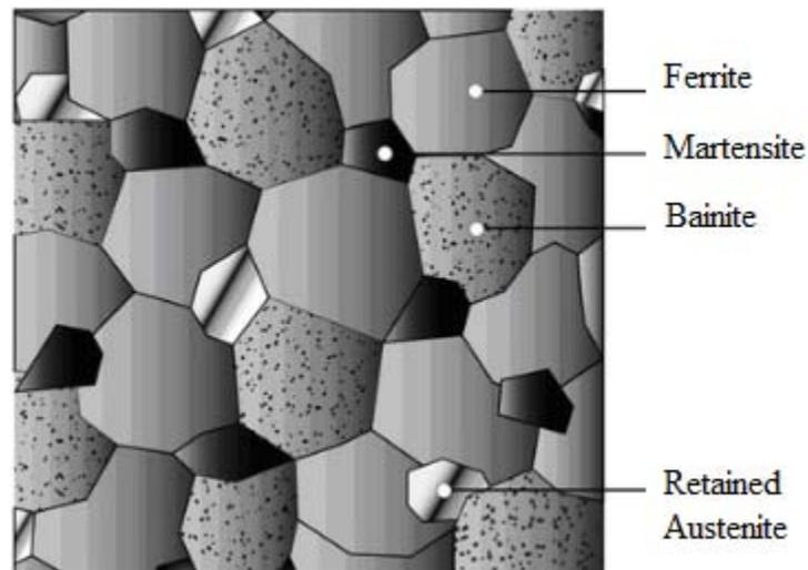
Figure 3.1 Schematic of TRIP steel showing the ferrite dominant matrix with phases of martensite, bainite, and retained austenite interspersed throughout.
