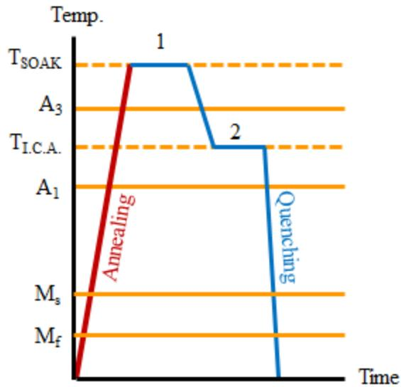
Figure 2.3 Heating/cooling schematic for the creation of DP steel.
