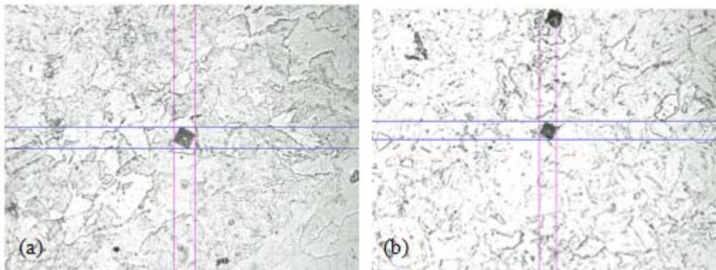
Figure 2.6 Vickers hardness indents showing indents on each phase of the steel.
