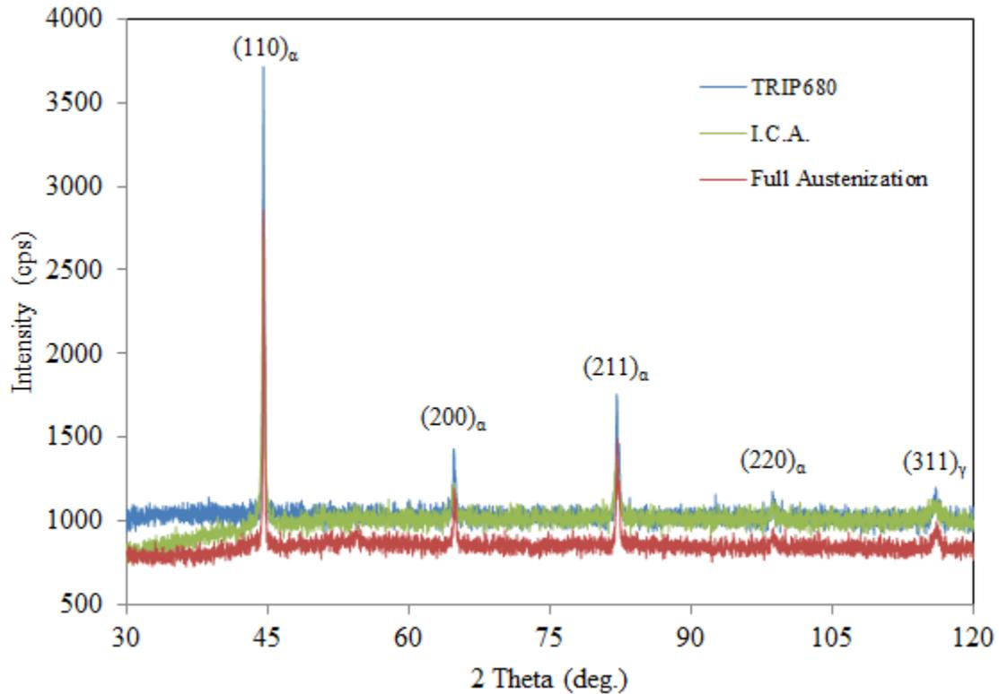
Figure 3.12 XRD Analysis of the TRIP steel series with the five major absorption peaks indexed.
