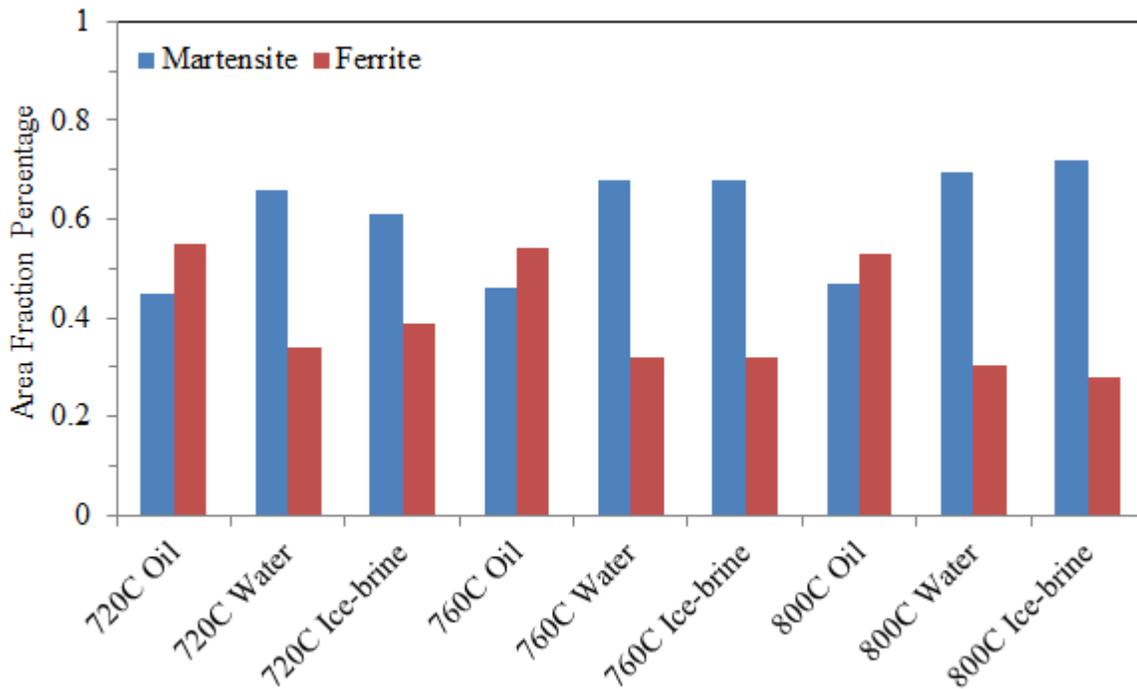
Figure 2.9 Area fractions of martensite and ferrite in different quenching cases.
