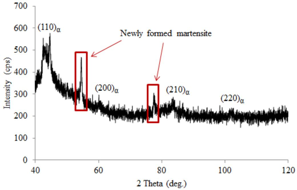
Figure 3.17 XRD Analysis of the TRIP steel series with the five major absorption peaks indexed.
