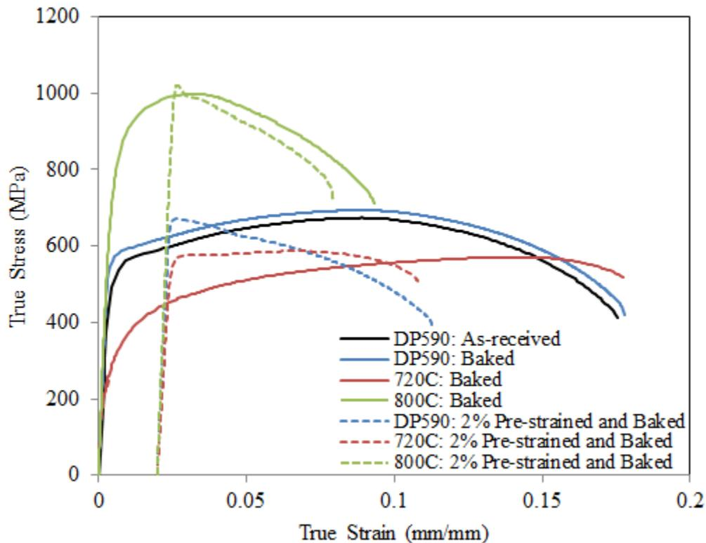
Figure 2.10 Quasi-static stress vs. strain results comparing the three different tempering cases at un-strained and 2% pre-strains tested at 0.01/s strain-rate.
