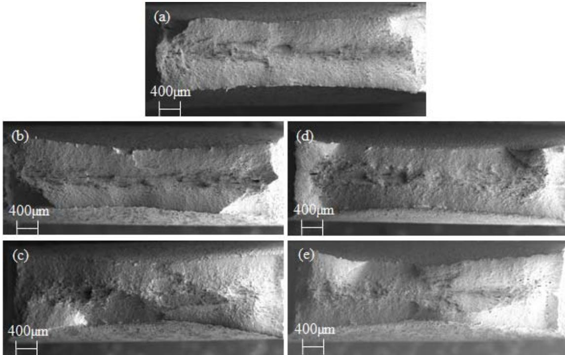
Figure 3.8 Fractography of specimens from quasi-static testing tested at 0.1/s strain rate.
