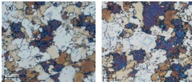
Figure 3.5 Optical microscopy showing Vickers indents on (a) bainite and (b) ferrite.
