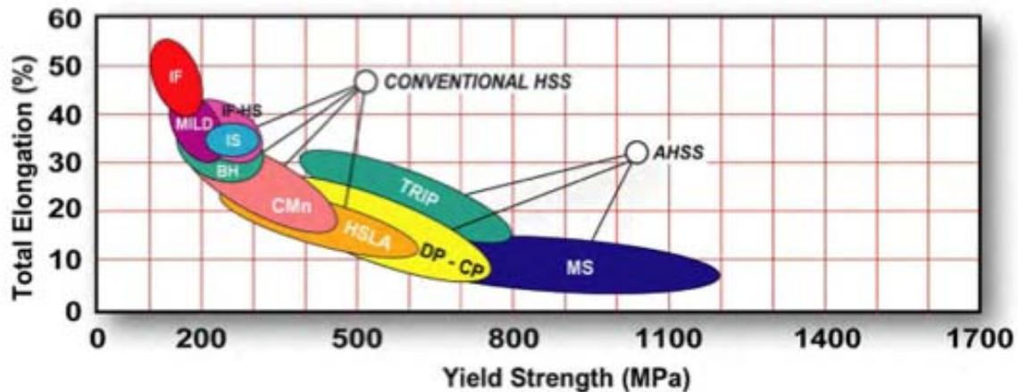
Figure 1.1 Depiction of AHSS (in color) in regard to strength and elongation compared to conventional steels (in grey).
