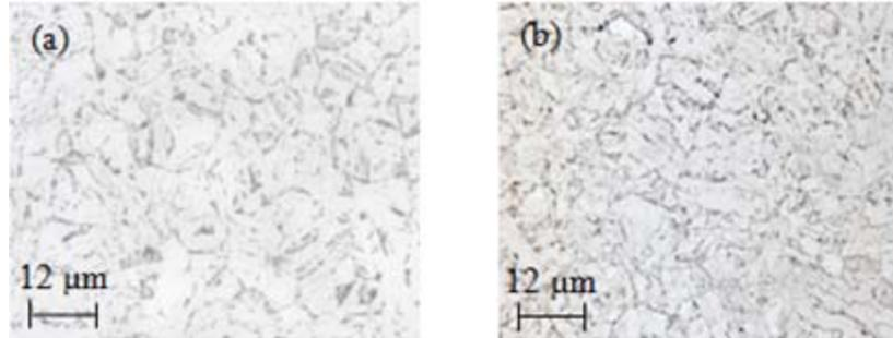
Figure 2.5 Microstructure of acquired DP steel.
