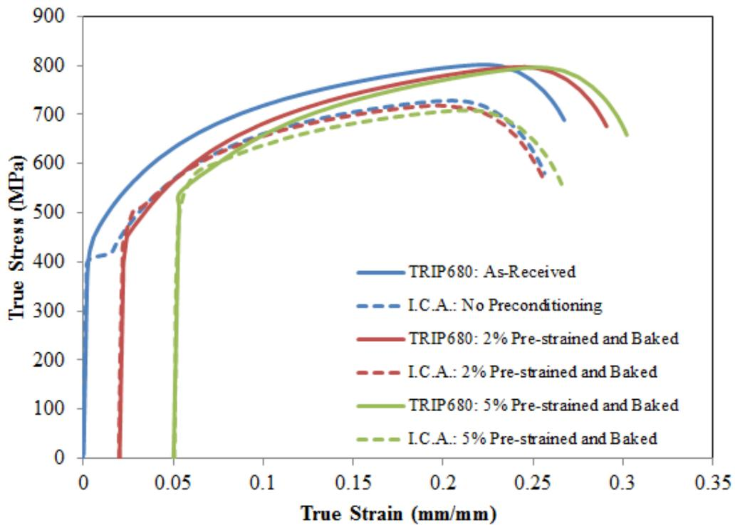
Figure 3.13 Quasi-static stress vs. strain results comparing the received TRIP680 to the I.C.A. series under three different preconditioning protocols.
