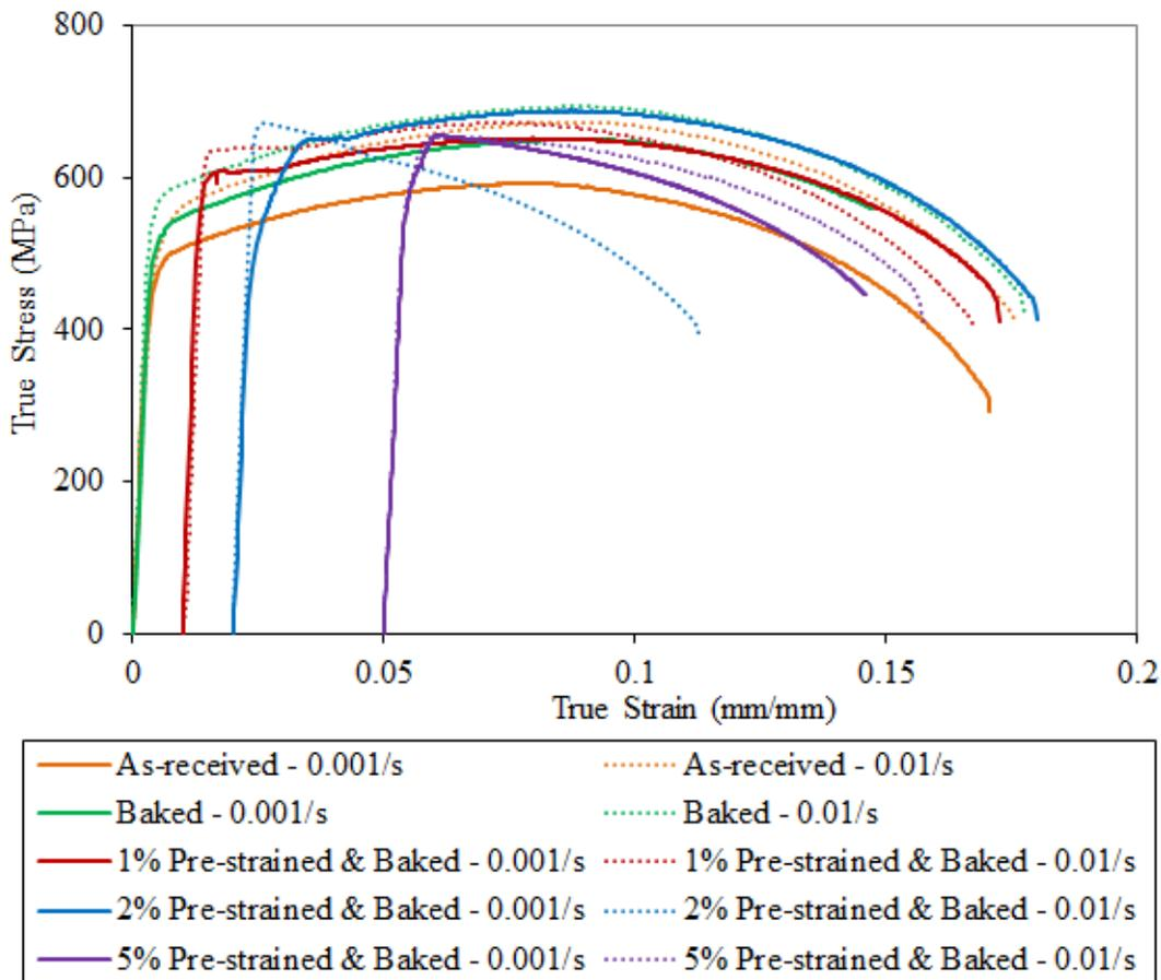
Figure 2.7 True stress vs. true strain curves from quasi-static tensile tests.
