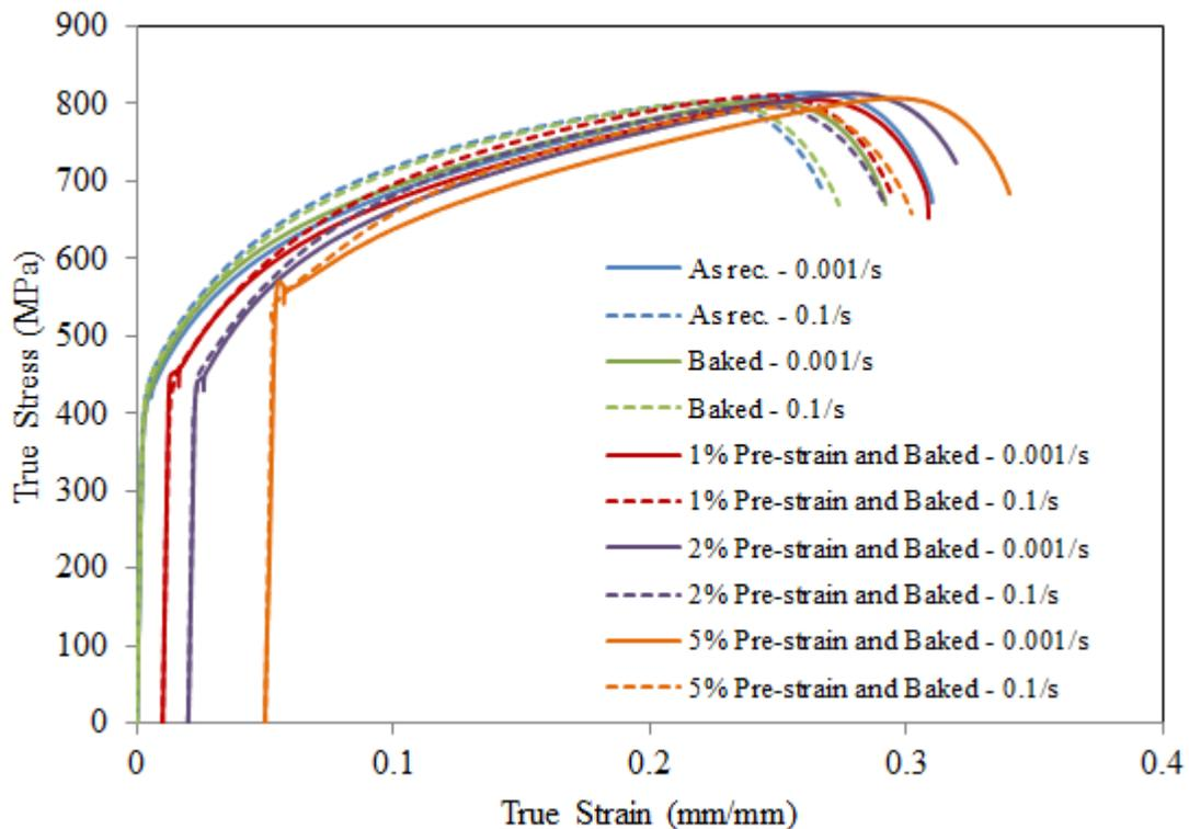
Figure 3.6 True stress vs. true strain curves resulting from quasi-static tensile tests.
