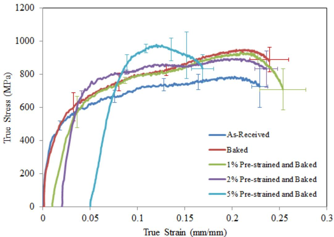
Figure 3.10 True stress vs. true strain graph resulting from high strain rate tensile tests.
