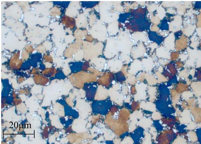
Figure 3.11 I.C.A. heat-treated TRIP steel showing the three phases of the steel: ferrite (tan and brown), bainite (blue), and retained austenite (bright white).
