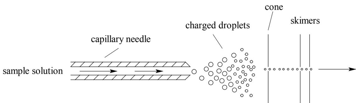
Figure 1 - 12. The diagram of electrospray ionization.
