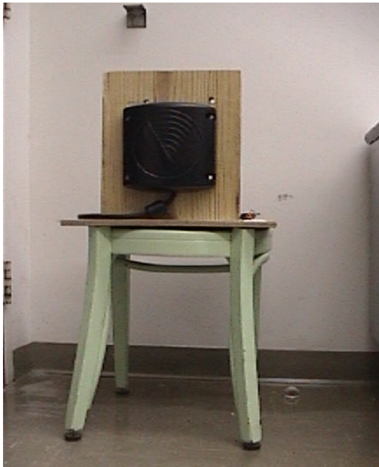
Figure 4.1: The mounting of the Preview sensor
