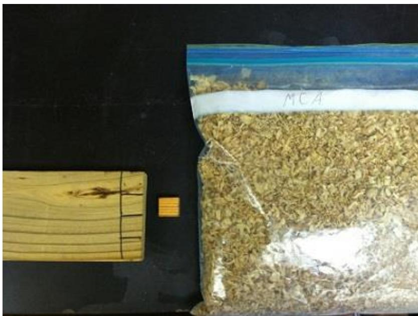
Figure 3.2 Before cut, after cut, and sawdust after being ground.
