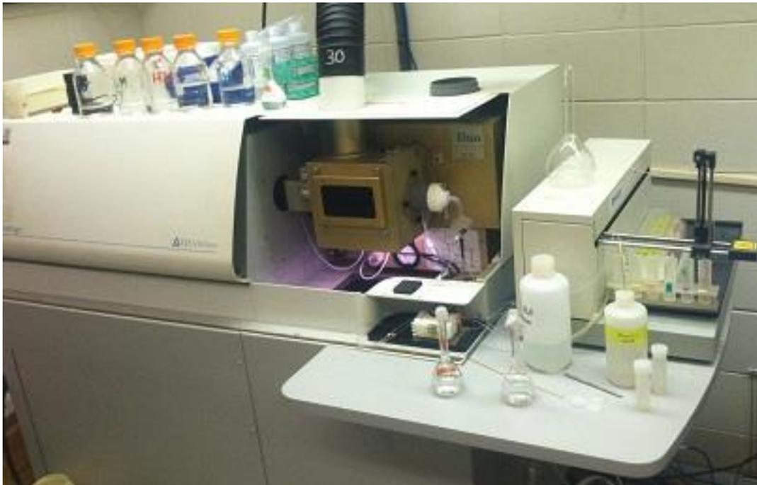
Figure 3.5 Inductively coupled plasma atomic spectroscopy.
