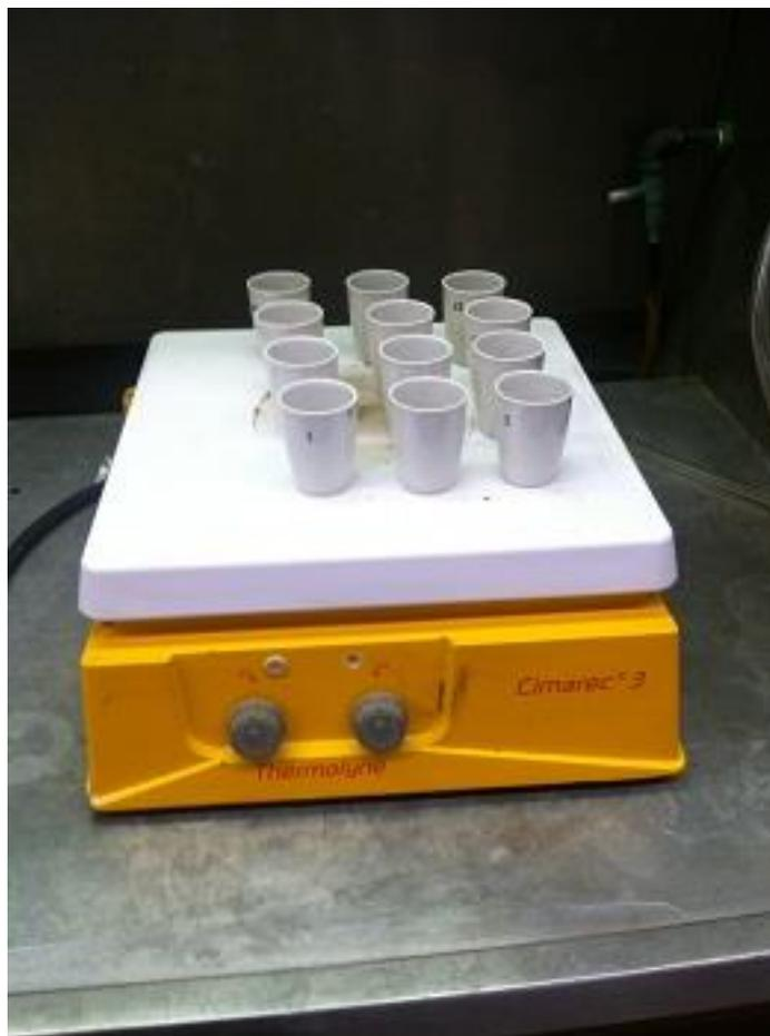
Figure 3.7 Samples on the hot plate.
