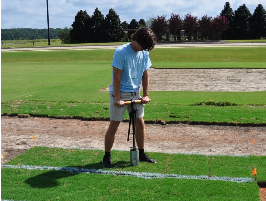
Figure 2.7 Core sample excavation
