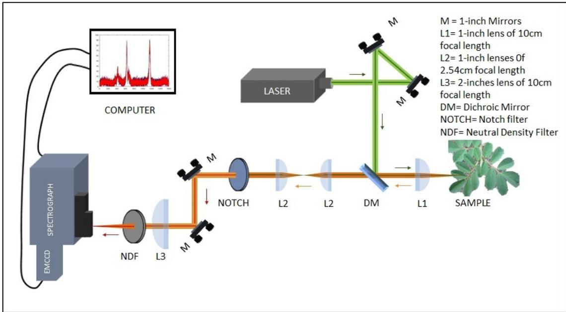
Figure 3.2 Experimental Raman setup
