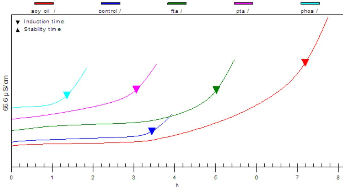
Figure 16 Rancimat graph illustrating the effect of treatments solutions with or without phosphate on the induction point (h) of catfish oil after one month storage time.
