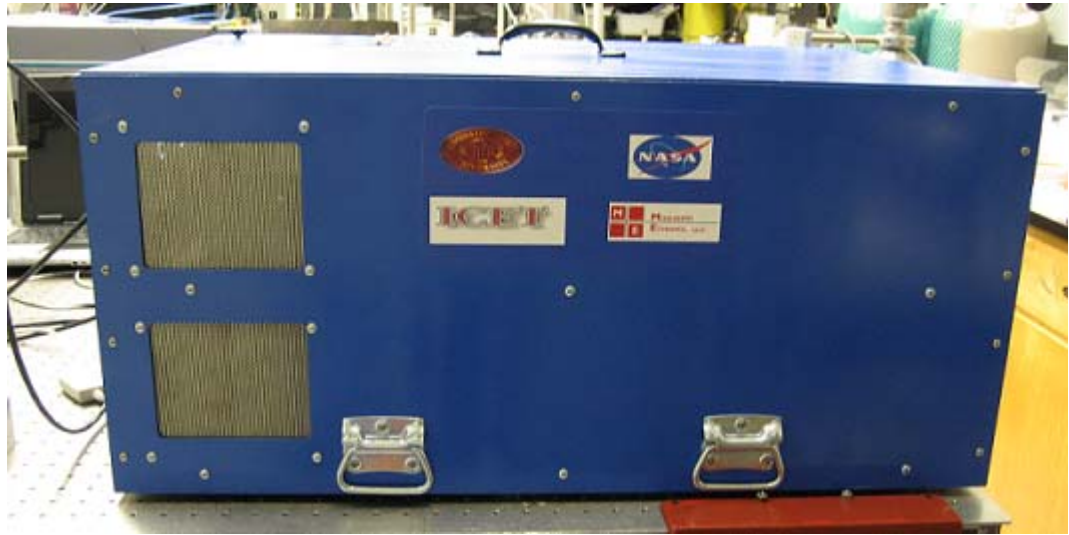
Fig. 3.14: Photograph of the complete integrated Raman sensor system.
