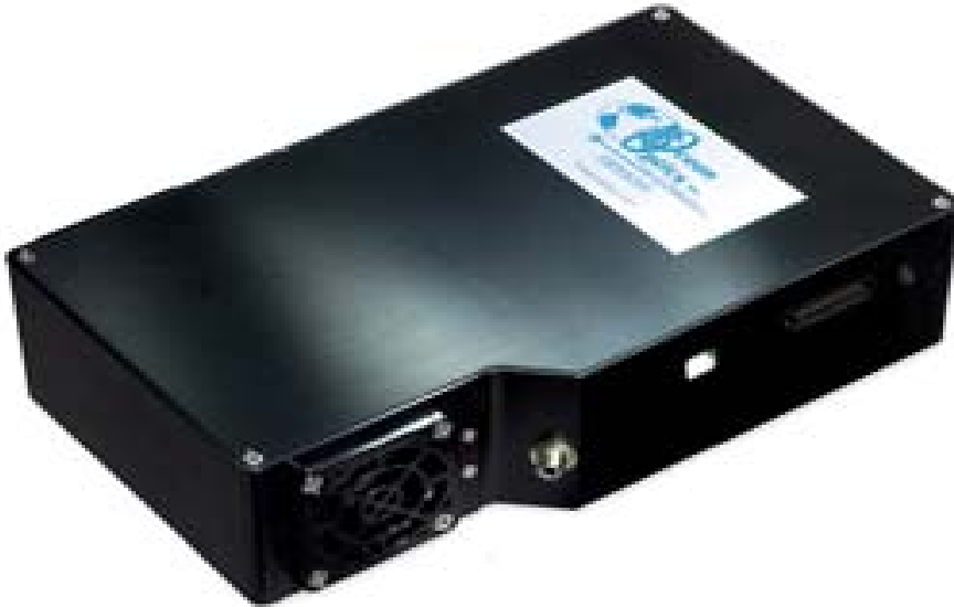
Figure 3.2: High-resolution Ocean Optics QE65000 scientific-grade spectrometer. 23
