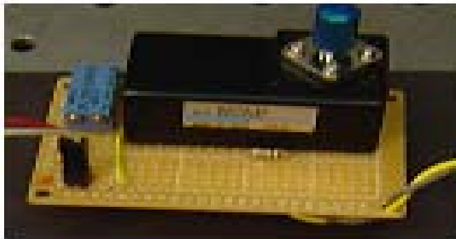
Figure 3.6 Photomultiplier tube (Hamamatsu Model H6776-20). 24
