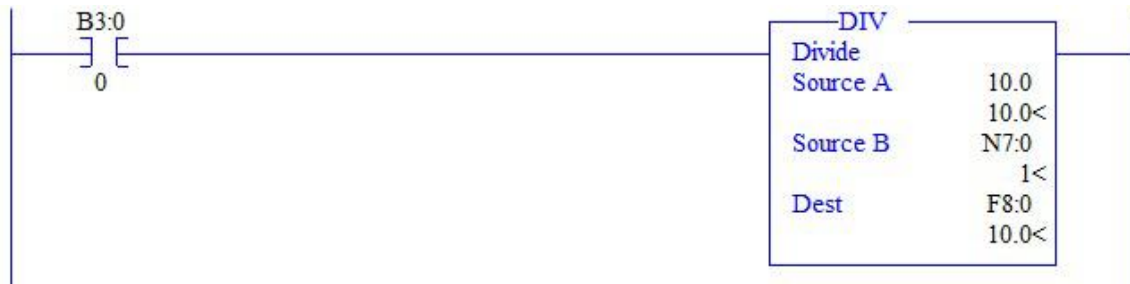
Figure 3.2 PLC Ladder Rung and Text Representation
