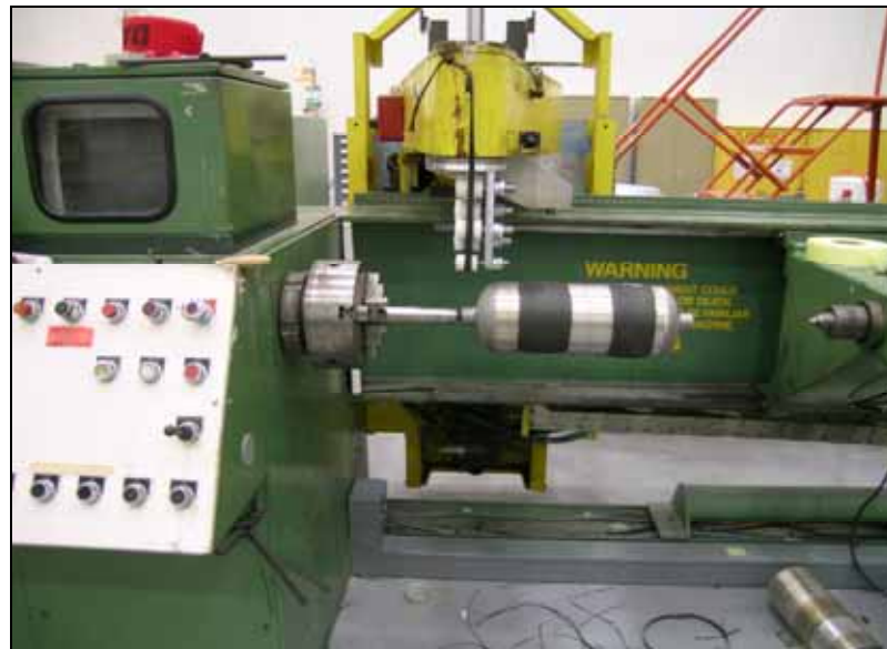
Figure 4.5 aluminum mandrel on filament winding machine
