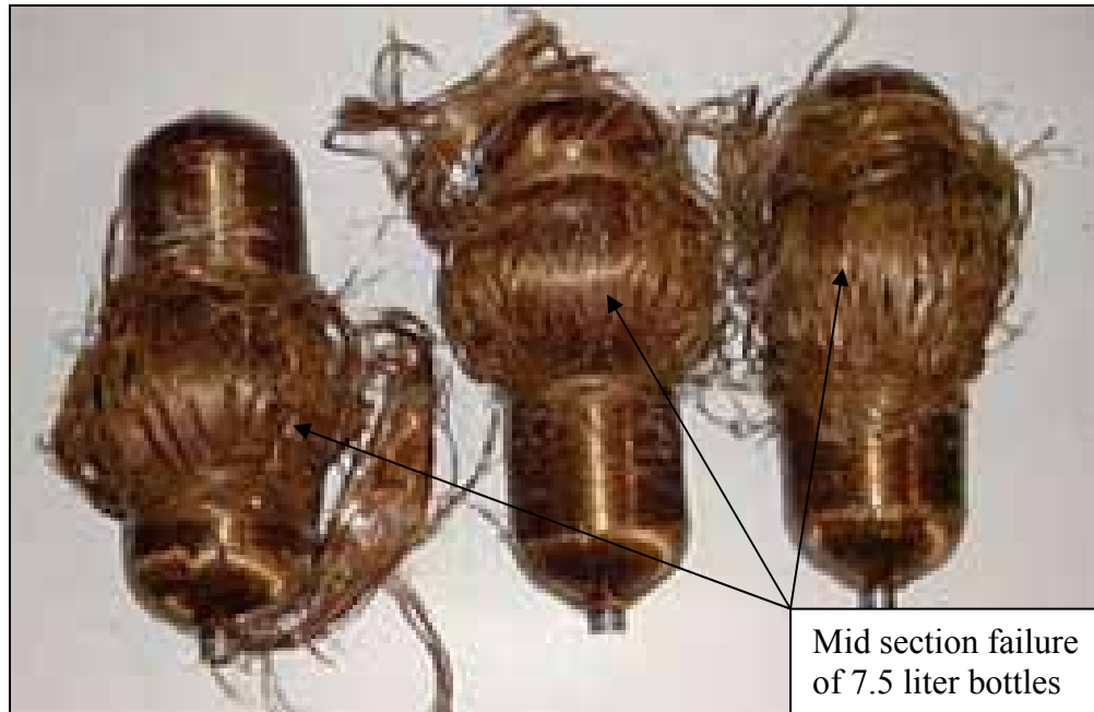
Figure 2.4 burst COPVs tested by Hypercomp Engineering Inc.
