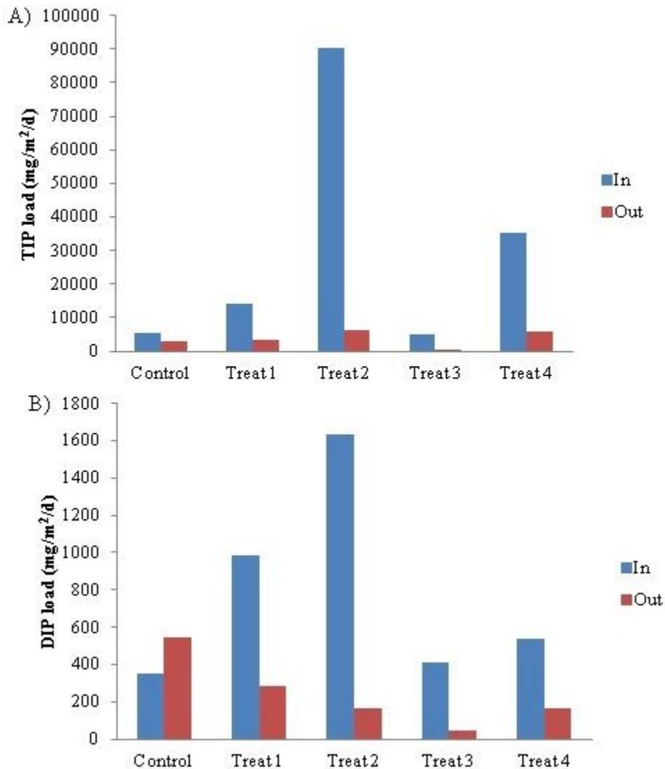
Figure 2.2 Aquaculture pond effluent phosphorus loads in and out of the vegetated ditch system.
