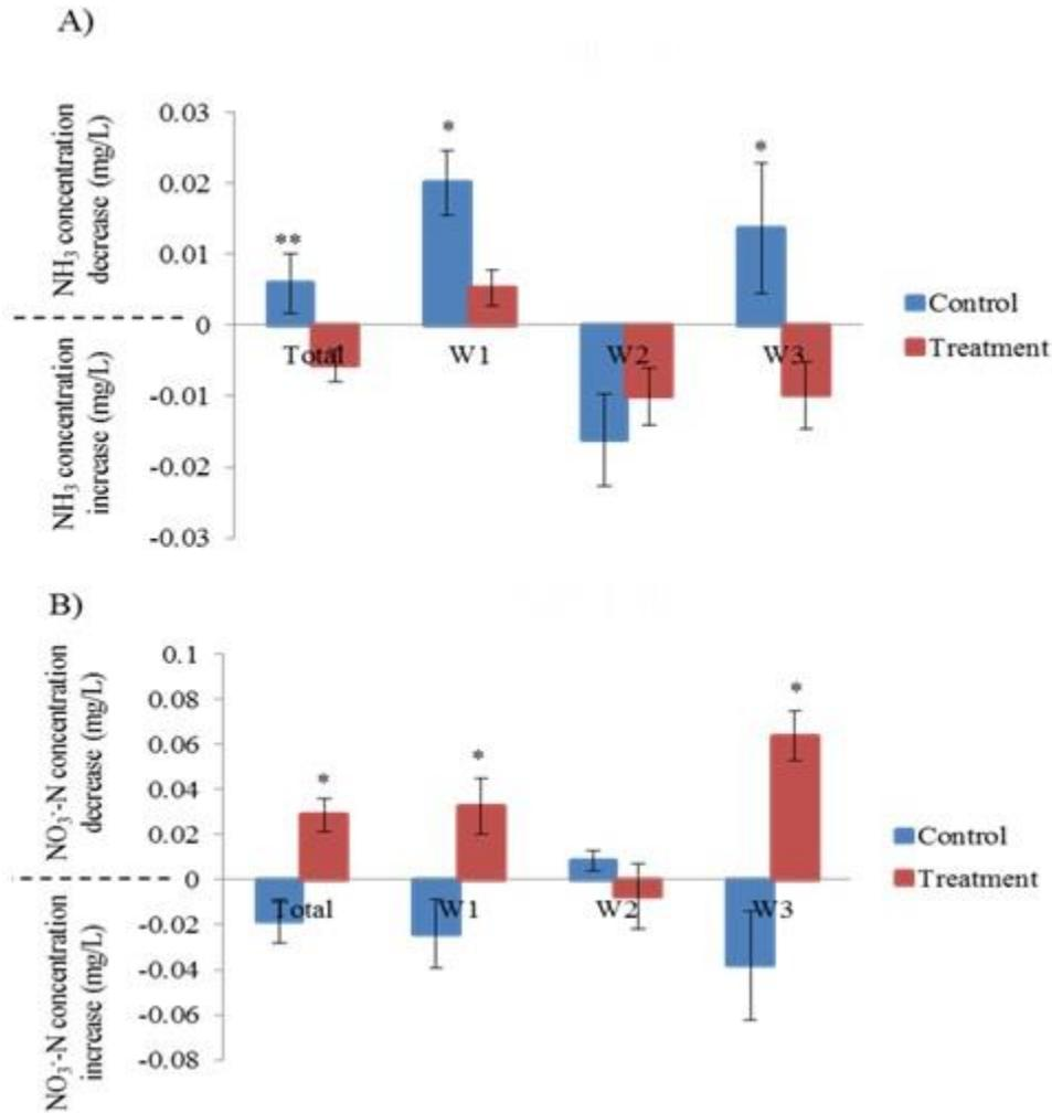
Figure 2.5 Mean nitrogen concentration reduction of aquaculture pond effluent in a vegetated ditch system fit with three consecutive low-grade weirs.
