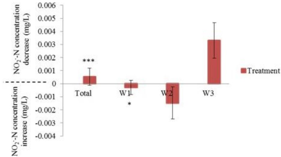
Figure 2.6 Mean nitrite concentration reduction of aquaculture pond effluent in a vegetated ditch system fit with three consecutive low-grade weirs.
