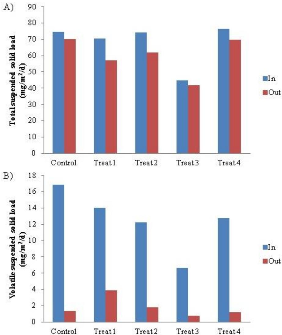
Figure 3.2 Aquaculture pond effluent suspended solids load in and effluent load out of a vegetated ditch system fit with three consecutive low-grade weirs.
