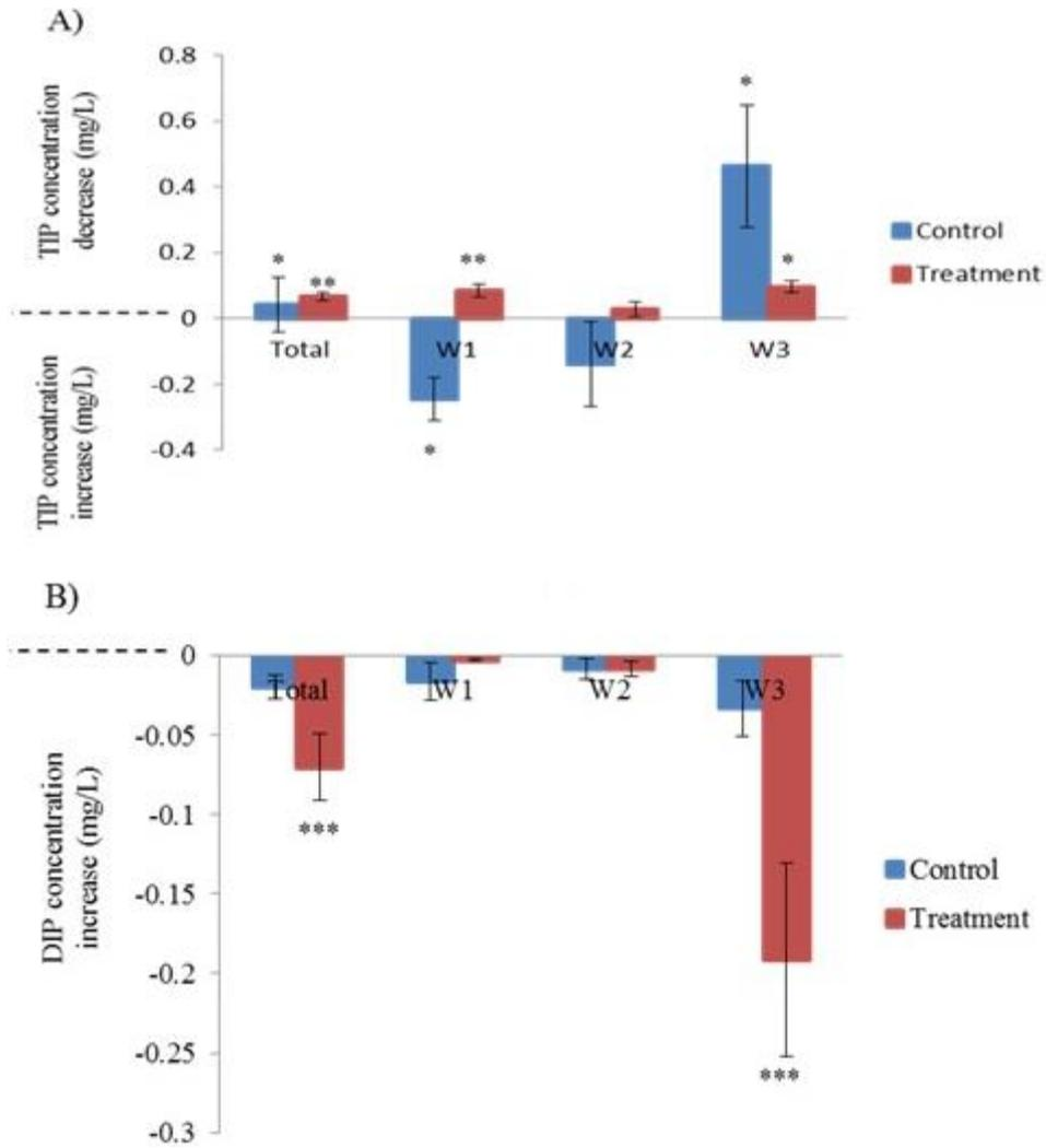
Figure 2.4 Mean phosphorus concentration reduction of aquaculture pond effluent in a vegetated ditch system fit with three consecutive low-grade weirs.
