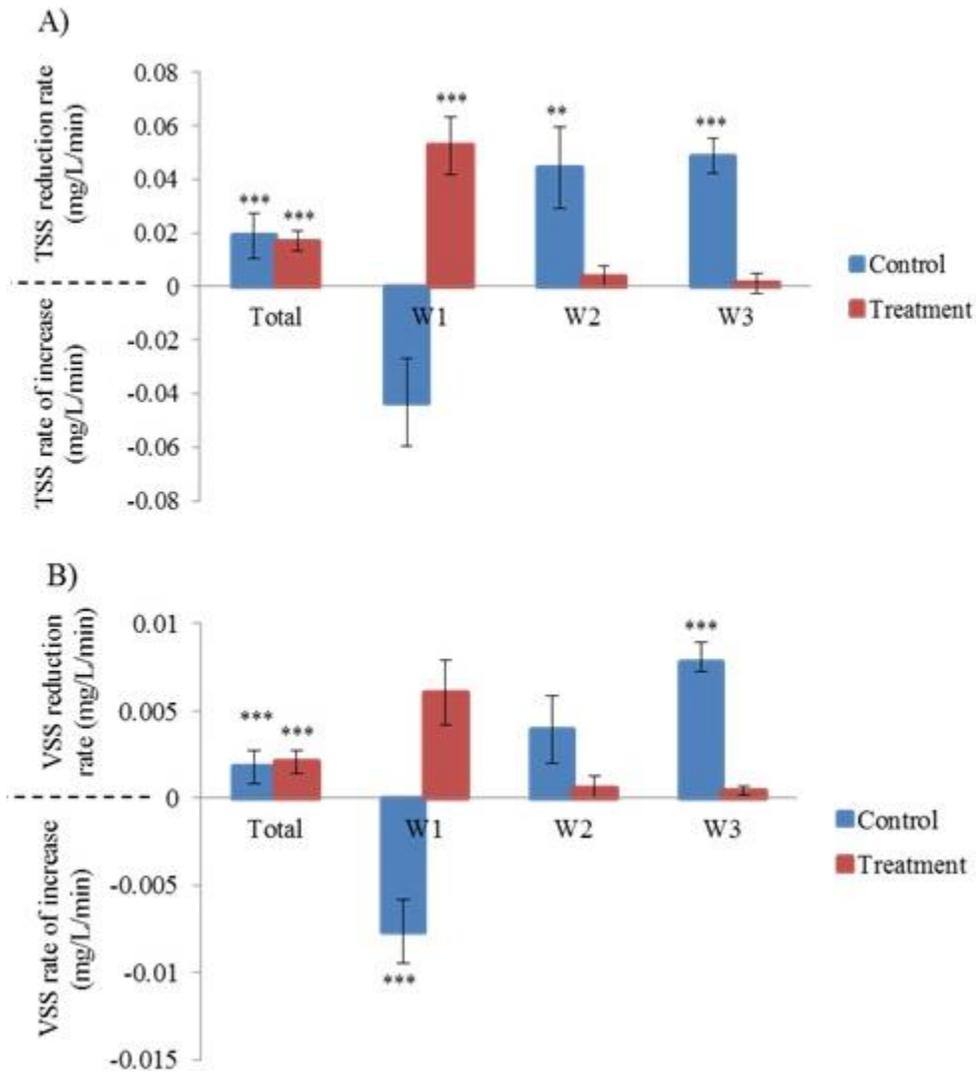
Figure 3.3 Mean suspended solids reduction rates of aquaculture pond effluent in a vegetated ditch system fit with three consecutive low-grade weirs.
