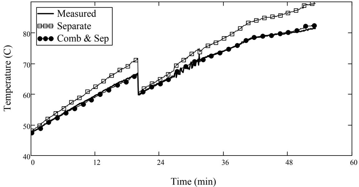
Figure 6.3 Connected model using coefficients from each of the parameter estimation methods (Recovery heat exchanger water outlet temperature,  $T_4$ )
