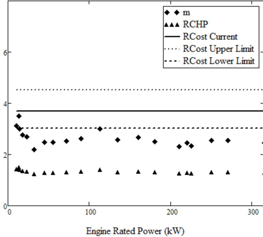
Figure 5.4 Parameters  $R_{cost}$ ,  $m$  and  $R_{CHP}$  versus PGU size
