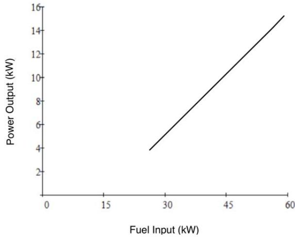
Figure 3.2 Engine Power Output Vs. Fuel Input (using data from engine manufacturer)
