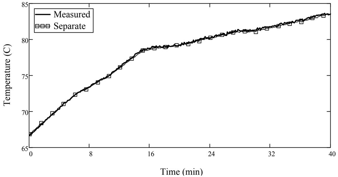
Figure 6.4 Single time step prediction where the parameters were estimated separately (Recovery heat exchanger water outlet temperature,  $T_4$ )
