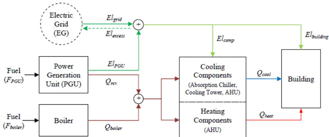
Figure 1.2 Schematic of CCHP system [Cho, 2009a]
