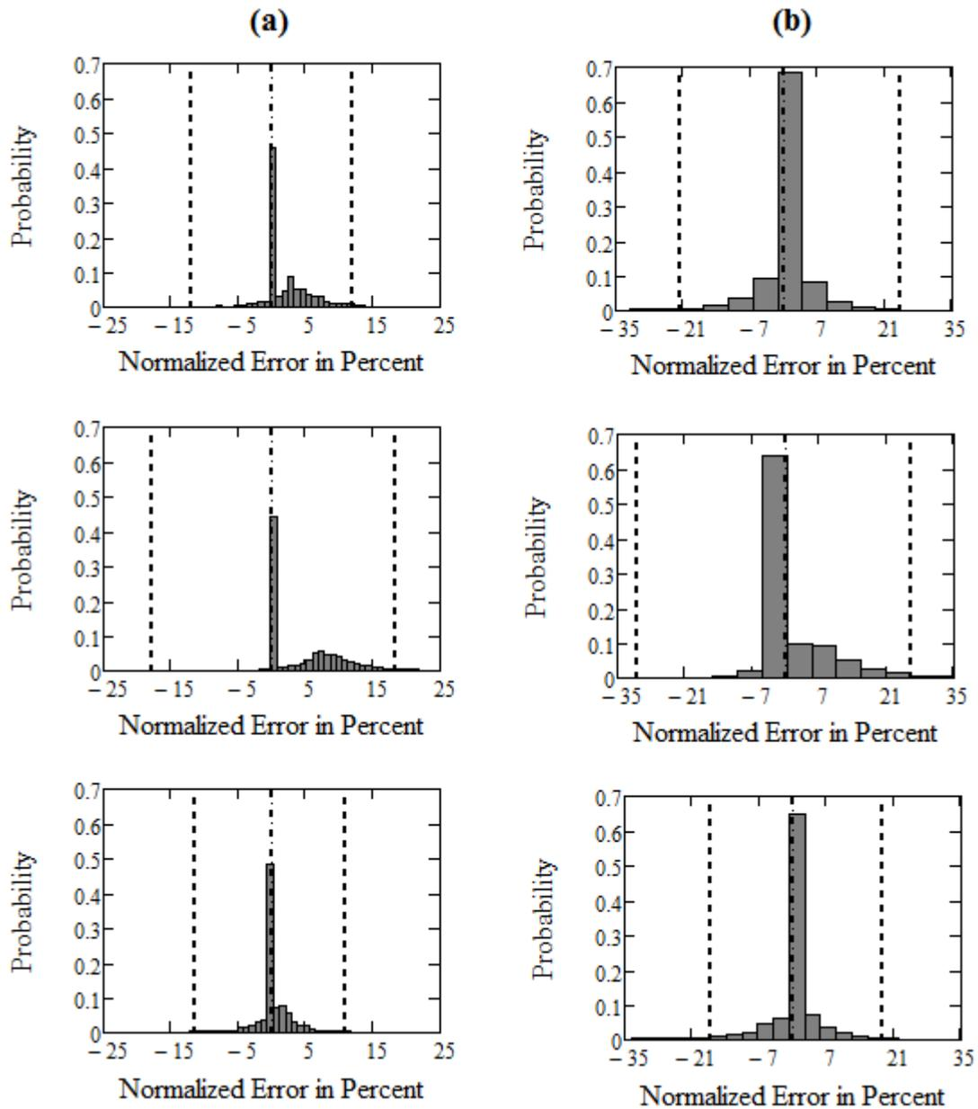
Figure 4.8 Histograms of errors for 30 degrees rotation for: (a) cooling at reference usage-density, +5% floor area (b) variable gas at -5% usage-density, +2% floor area.
