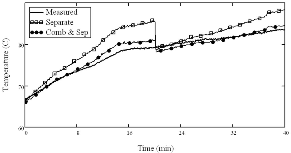
Figure 6.6 Example comparison of the methods for 20 minute prediction (Recovery heat exchanger water outlet temperature,  $T_4$ )
