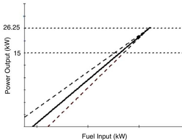
Figure 3.3 Engine power output uncertainty range (exaggerated for visualization)
