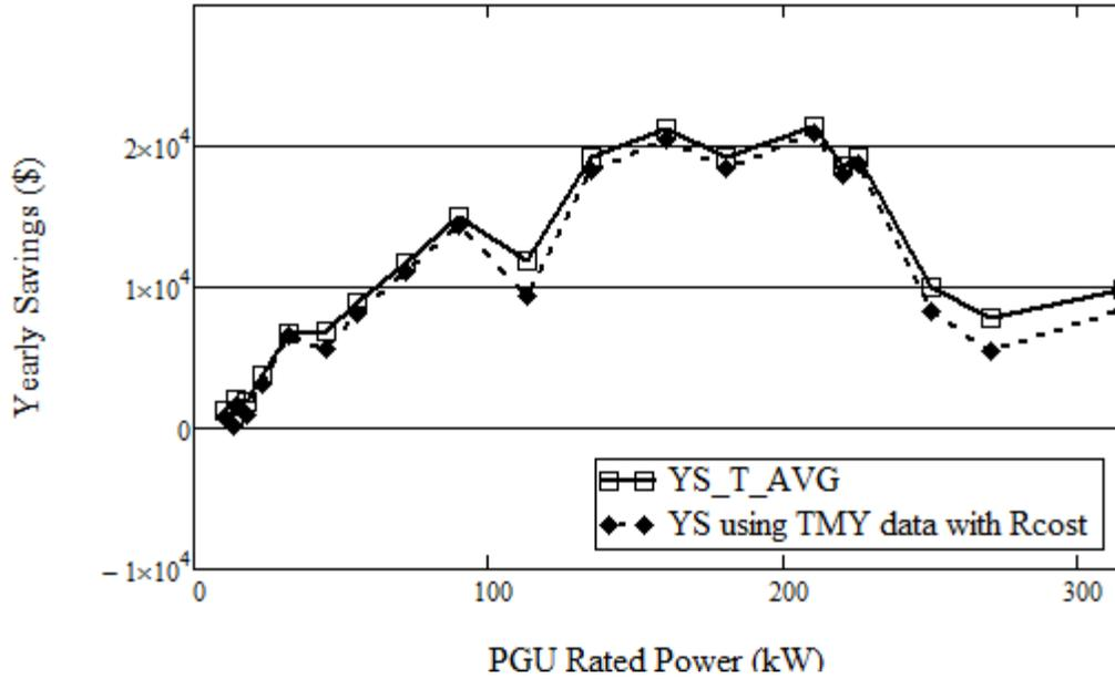
Figure 5.6  $YS_{T\_AVG}$  and YS using TMY data with the current cost ratio
