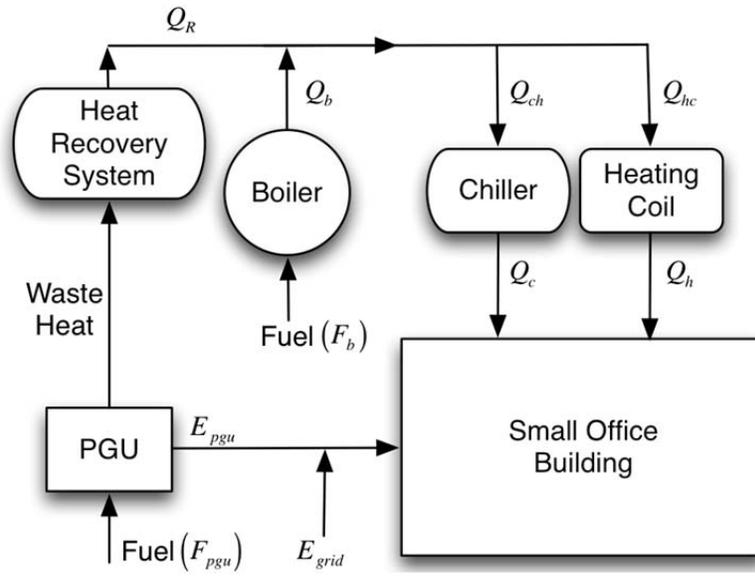
Figure 3.1 Schematic of a CCHP system
