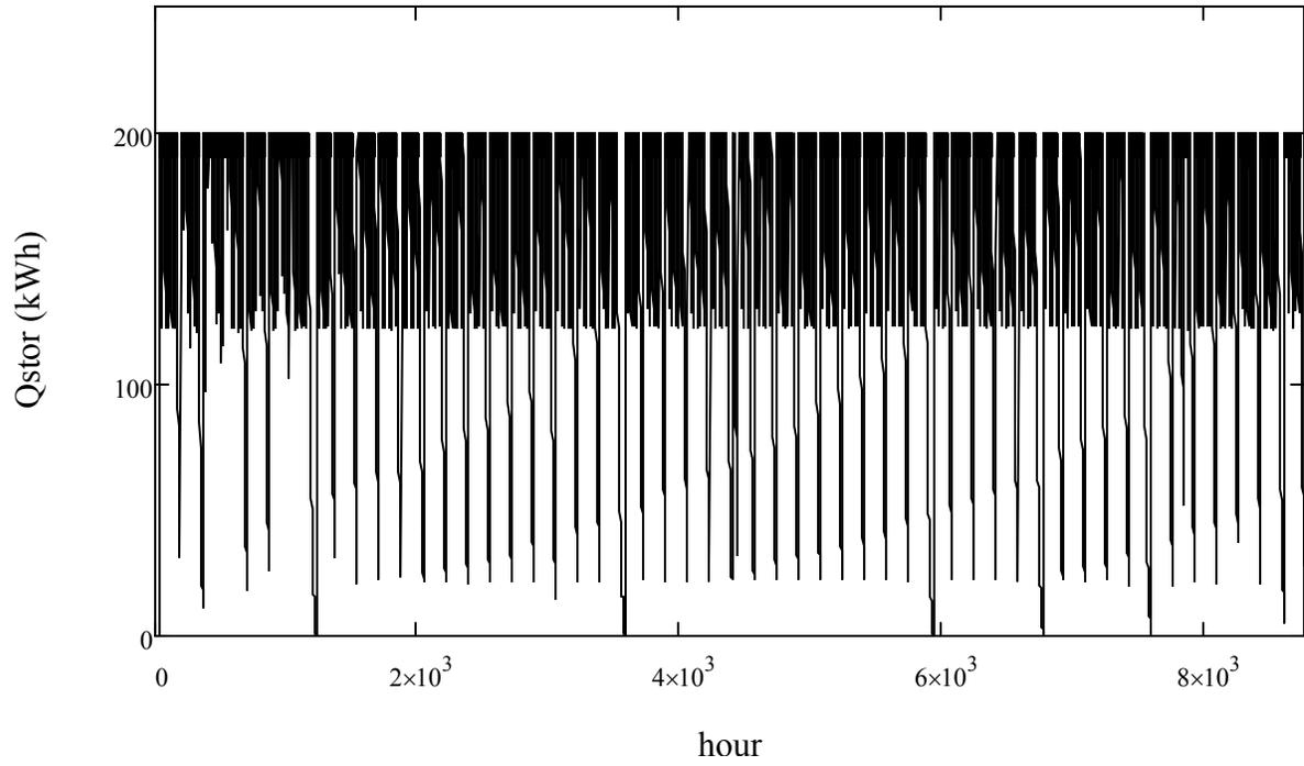
Figure 5.7 Hourly  $Q_{stor}$  for the 210 kW PGU with  $R_{costU}$  for weather data from 1997
