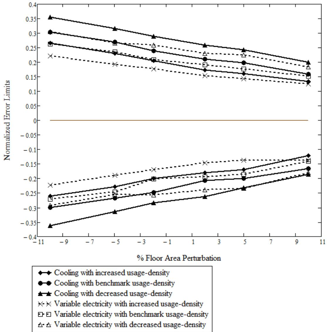
Figure 4.5 Cooling and Variable Electricity Error Limits for 60 Degree Rotation
