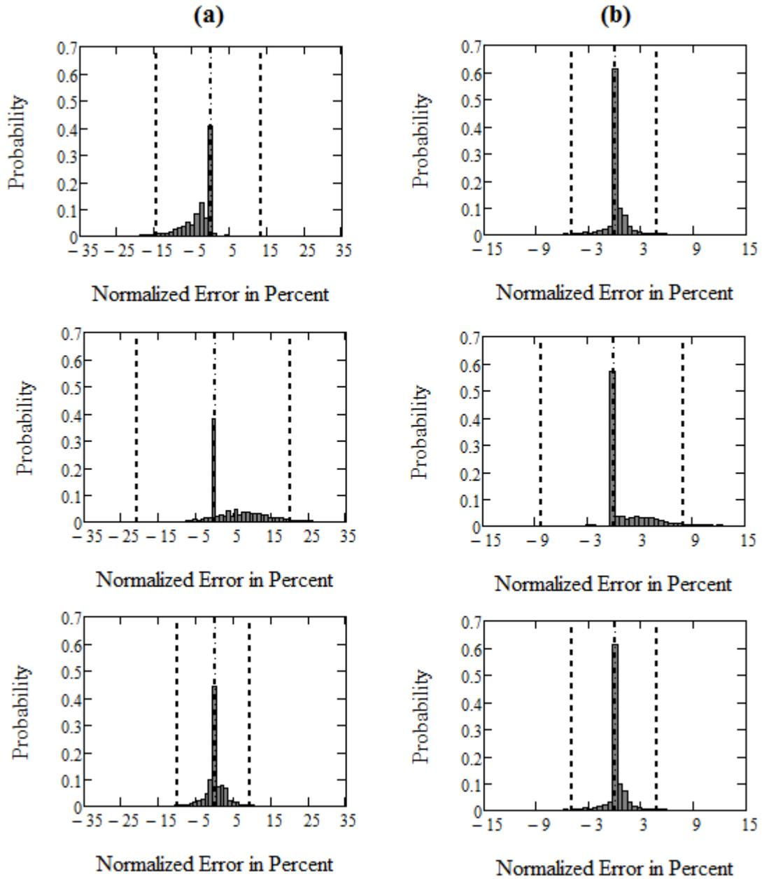
Figure 4.7 Histograms of errors for 0 degrees rotation for: (a) variable electricity at +5% usage-density, +10% floor area (b) variable gas at -5% usage-density, +5% floor area.
