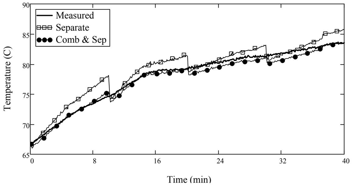
Figure 6.5 Example comparison of the methods for 10 minute prediction (Recovery heat exchanger water outlet temperature,  $T_4$ )
