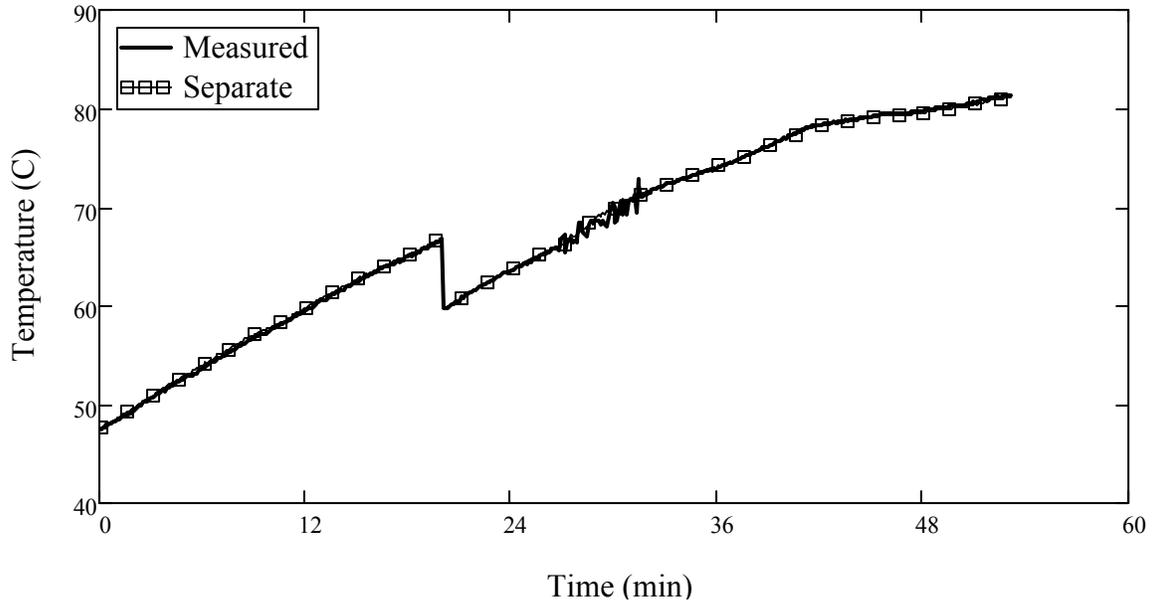
Figure 6.2 Single time step prediction where the parameters were estimated separately (Recovery heat exchanger water outlet temperature,  $T_4$ )
