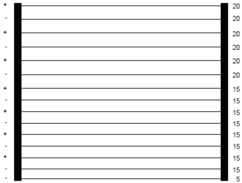
Figure 2.2 Wire spacing (cm) of a 15-strand high-tensile electric fence (height = 2.5 m) with alternating positive (+) and negative (-) wires constructed around the Samuel Roberts Noble Foundation Wildlife Unit in Oklahoma.
