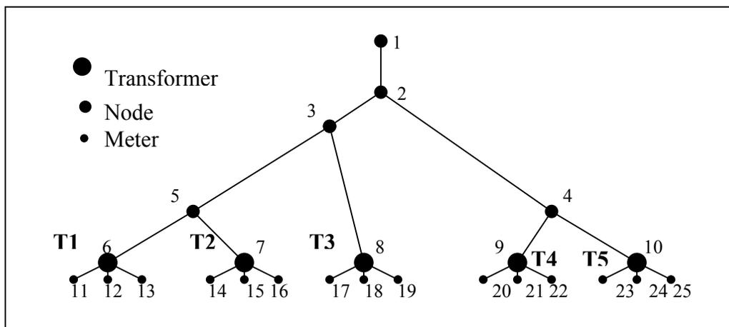
Figure 5.2 Representation of a Distribution Network
