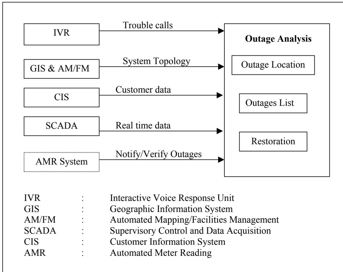
Figure 1.3 Structure of an Outage Management System
