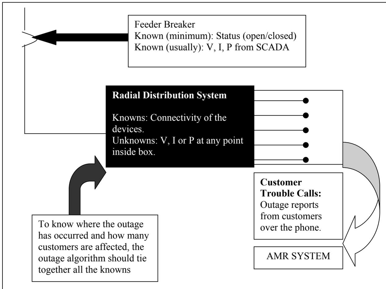
Figure 1.2 Available information in a typical distribution system [2]
