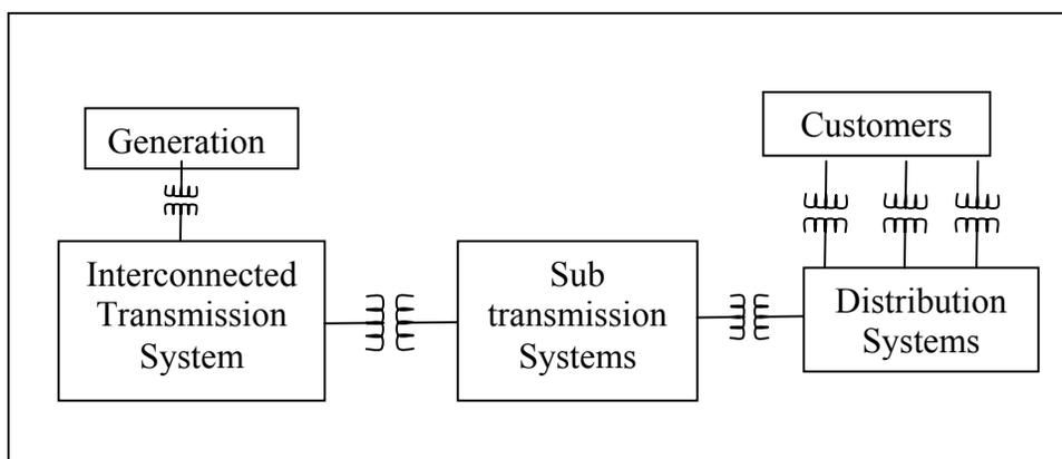
Figure1.1 Typical Power System Components [1]
