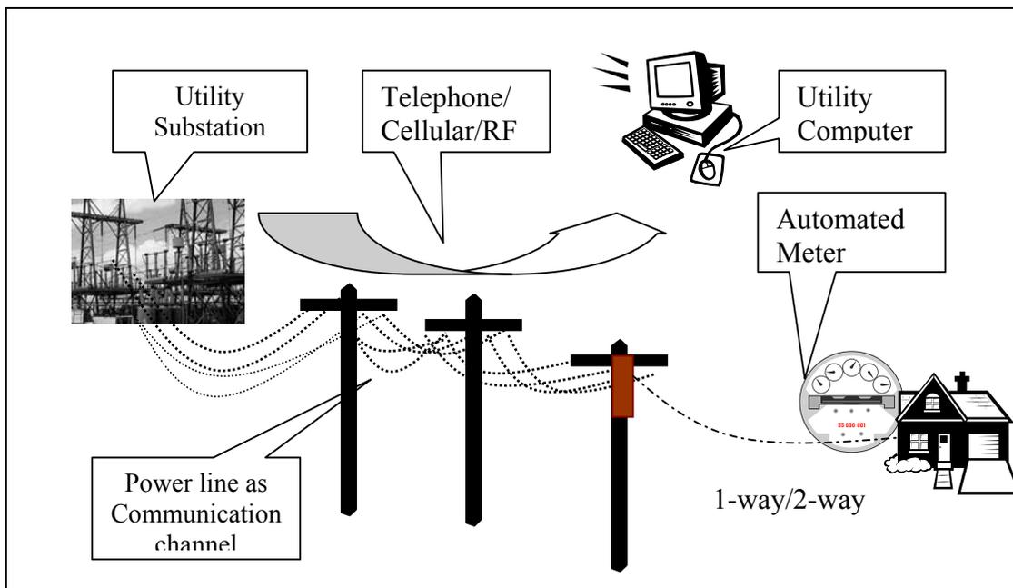
Figure 2.3 Flow of data in Powerline Carrier AMR Systems
