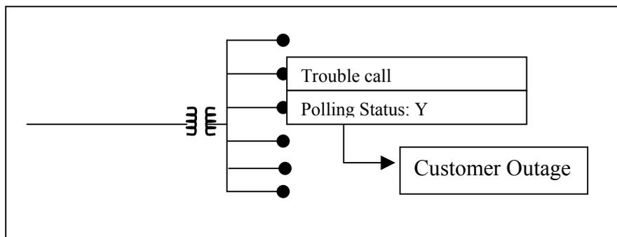
Figure 5.8 The case of a single customer outage
