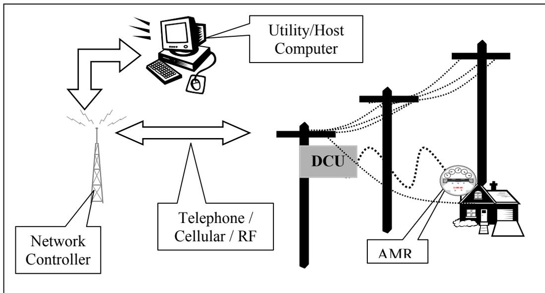
Figure 2.2 Flow of data in radio based AMR systems
