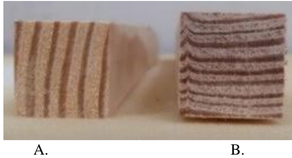
Figure 2.4 Specimen A was loaded on the radial face and specimen B was loaded with the tangential face nearest to the pith.
