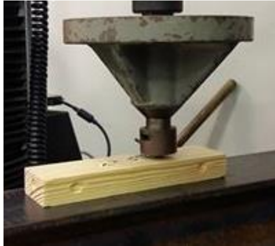
Figure 2.7 Janka ball side hardness test setup.
