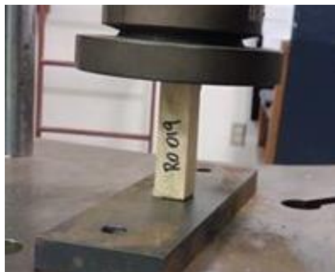
Figure 2.5 Compression parallel to the grain test setup.
