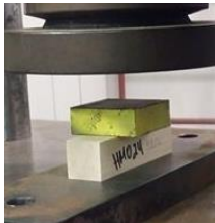
Figure 2.6 Compression perpendicular to the grain test setup.
