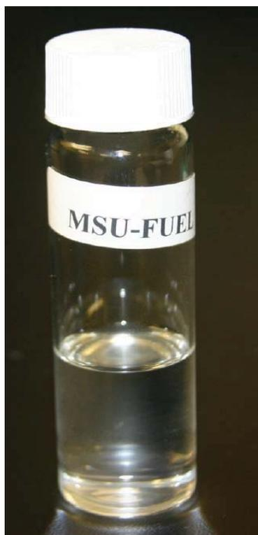
Figure 3.8 Water clear hydrocarbon mix produced by HC process using MSU-2 catalyst.
