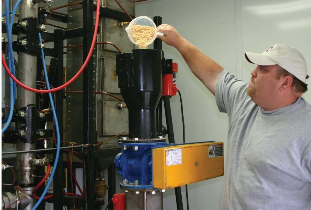
Figure 2.1 Production of bio-oil by auger reactor technology at MSU; wood particle in feed shown.
