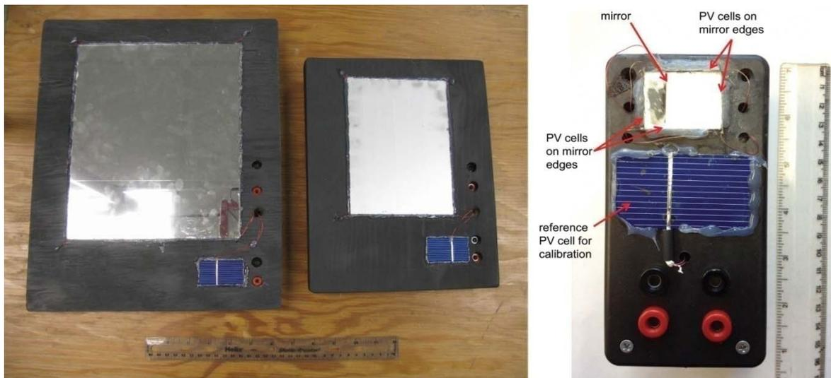
Figure 2 Prototype concentrators; large, medium, and small, from left-to-right.
