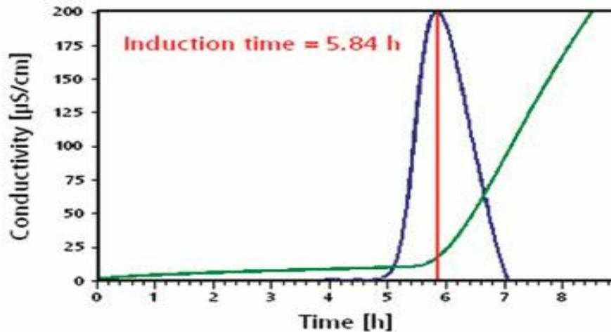
Figure 3. Calculation of inflection point of the conductivity vs. time curve for oil stability index, OSI (Steinbach, 2007)
