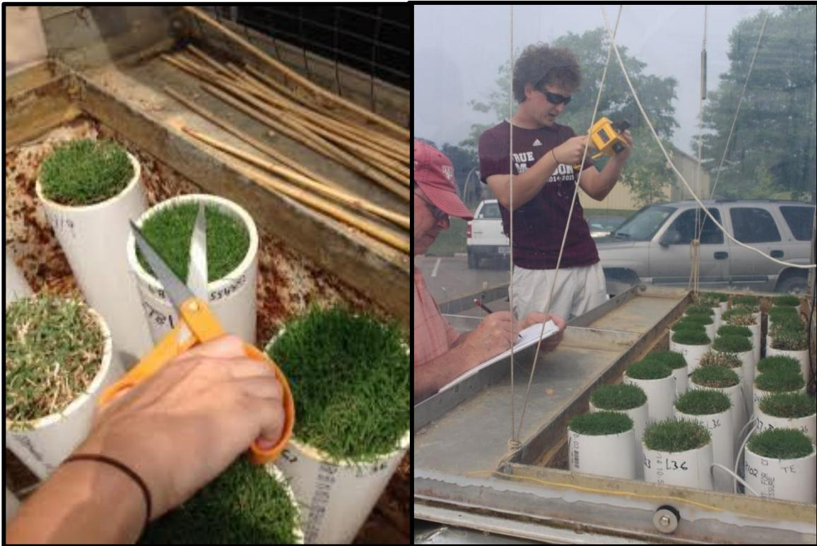
Figure A.2 Harvesting clippings using scissors and a PVC guard cut to a desired height and the collection of relative chlorophyll index data using the CM 1000 handheld reflectance meter.
