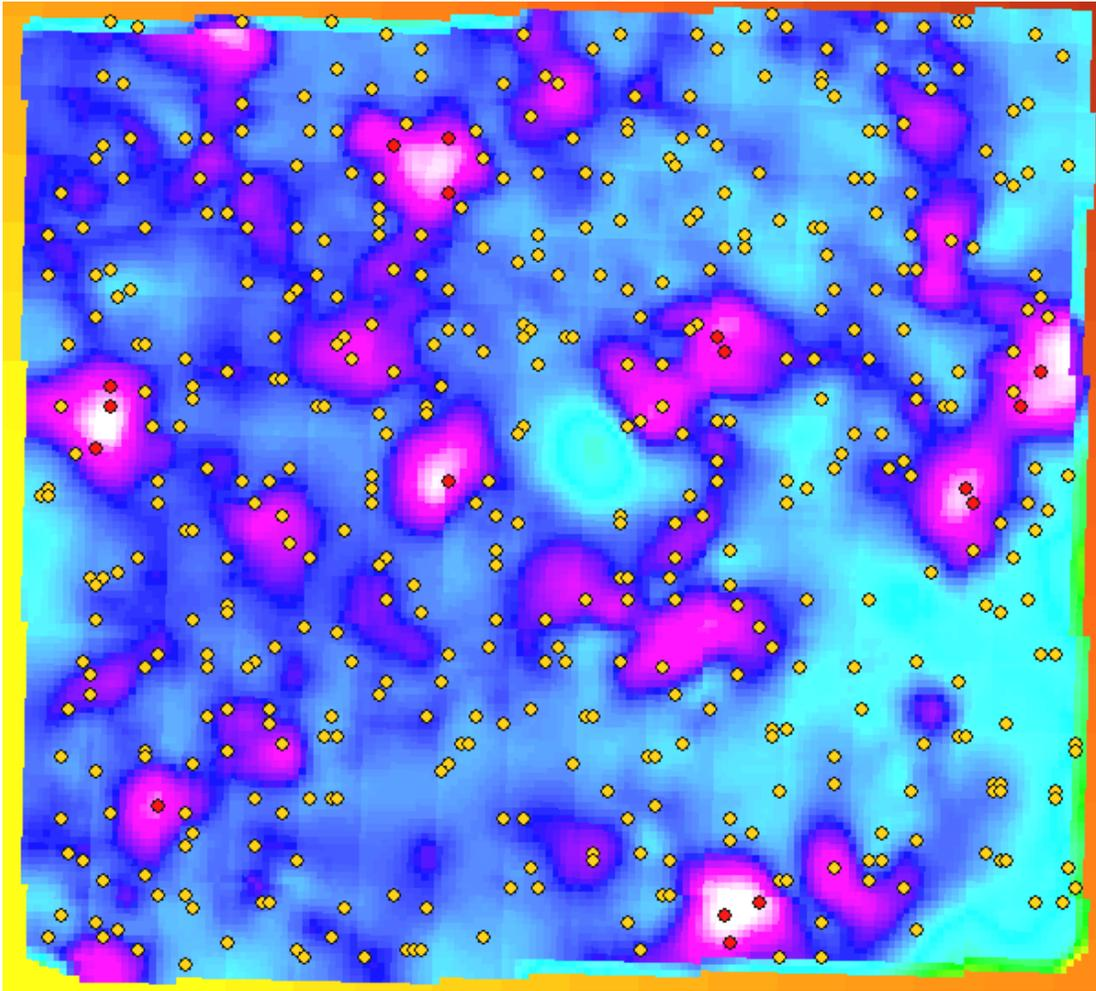
Figure 2.3 A small subset of the initial bare ground surface viewed with LiDAR Analyst in ArcMap. The dots shown are the predicted LiDAR ground points. The red dots are predicted ground points that were greater than 1.5 meters different from the 10m DEM. These points were removed before final interpolation.
