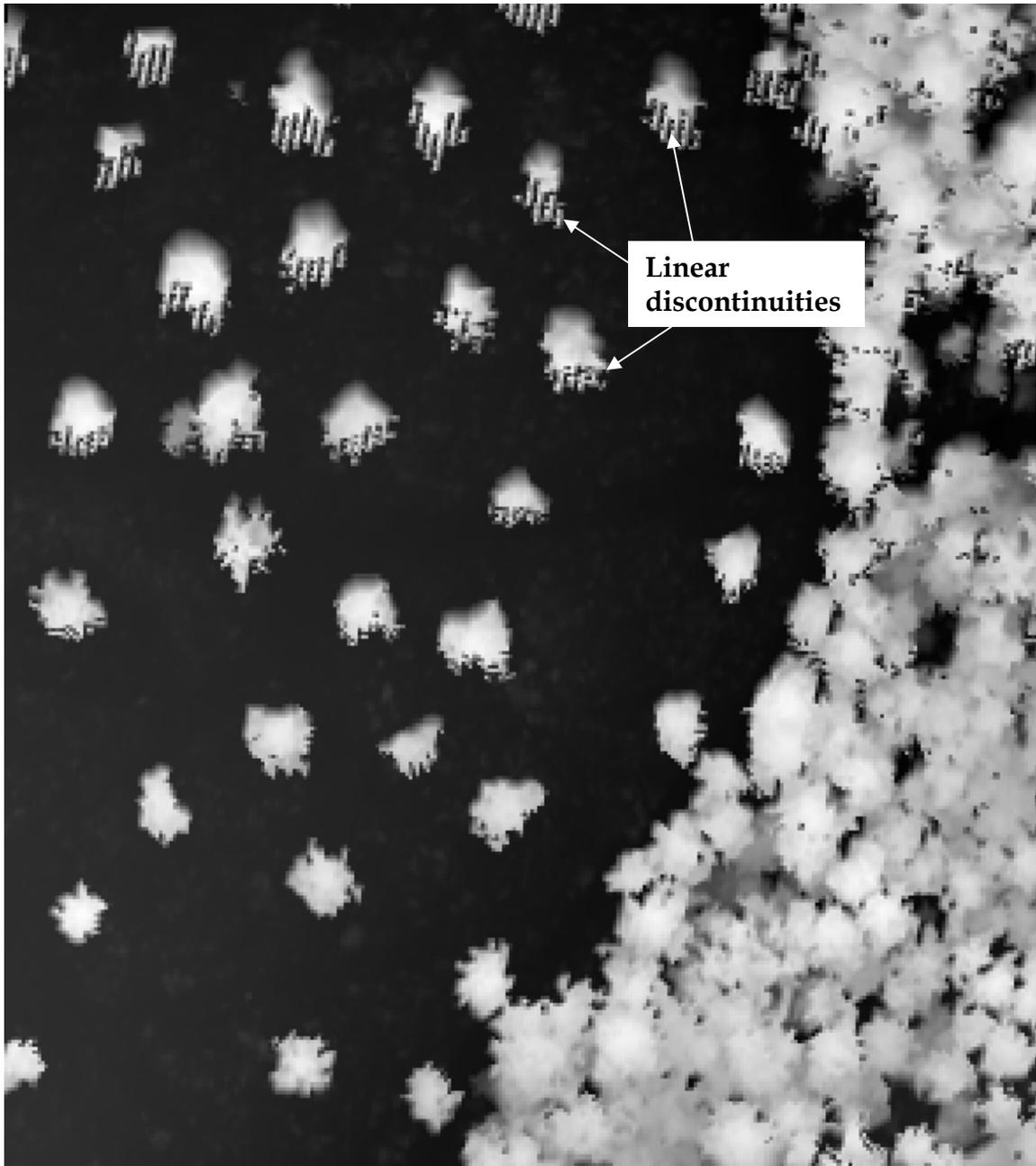
Figure 4.1 Canopy surface of the northern portion of an EW flightline showing linear discontinuities pointing toward nadir (bottom of image). Area being viewed is isolated seed trees on left and closed canopy on the right. The gray tones in this response surface represent relative heights of the vegetation.
