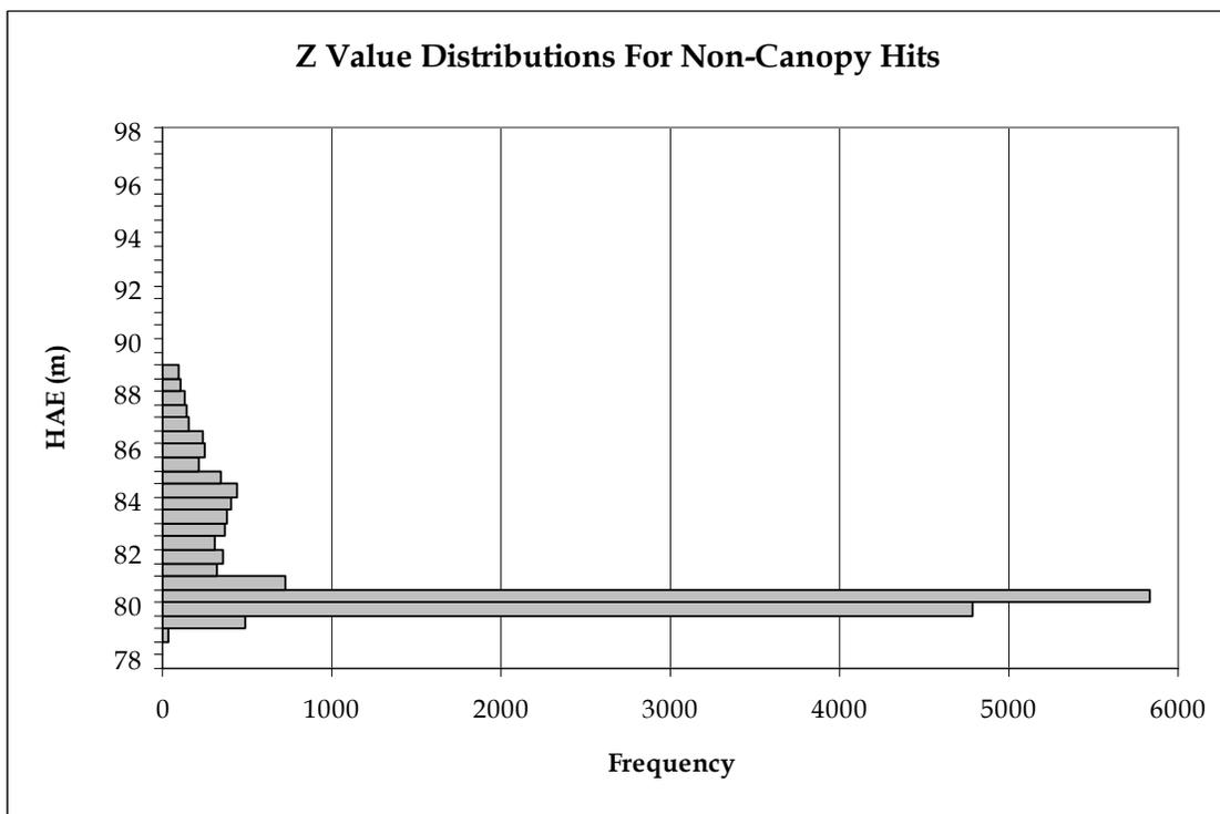
Figure 2.2 Distributions of Z values in height above ellipsoid (HAE) before (above) taking out LiDAR canopy hits and after (bottom) taking out canopy hits (includes mid- and understory hits).
