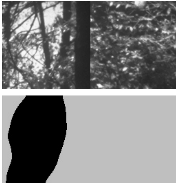
Figure 25. Another example segmentation with the Gabor feature design. The left half image is a typical “bgsky” (background sky) block, and the right half is a “bush” block. In the segmentation image, the black region stands for hypotheses for the “bgsky” category, while the grey color is used for “bush.” The pixel classification error rate was 22.0%.
