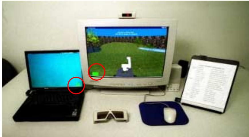
Figure 4. Photograph of virtual and real-world battery displays for monitoring tasks (see shapes inside superimposed circles).
