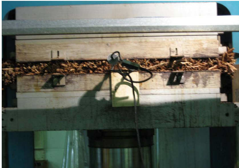
Figure 3.6 Scrim Material Being Pressed Into Board
