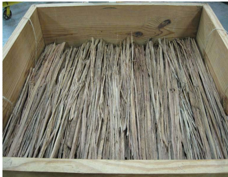
Figure 3.2. Board Being Formed in Same Grain Direction
