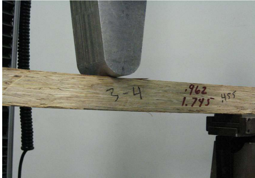
Figure 4.2. Specimen Being Tested in Joist/Beam Orientation.
