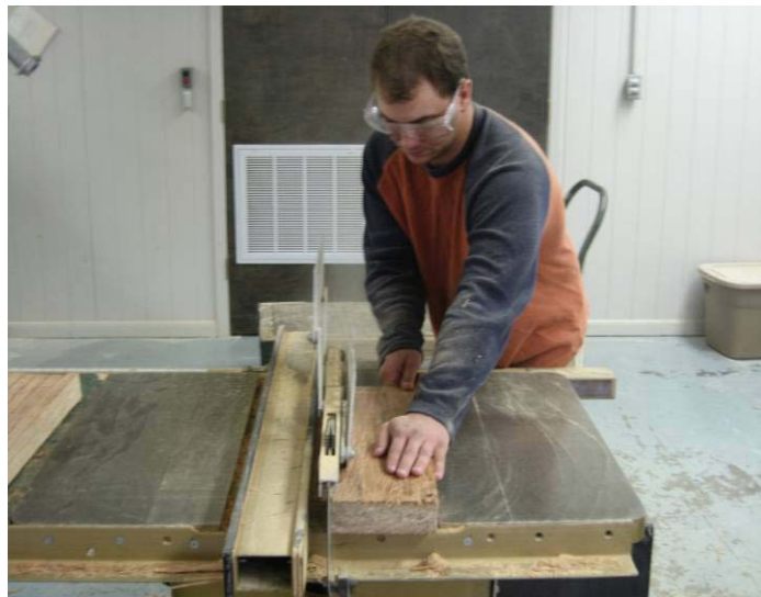
Figure 4.1. Sawing Specimen to Length and Width
