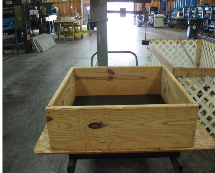
Figure 3.1. 34"x34"x12" Box with Bottom caul Plate
