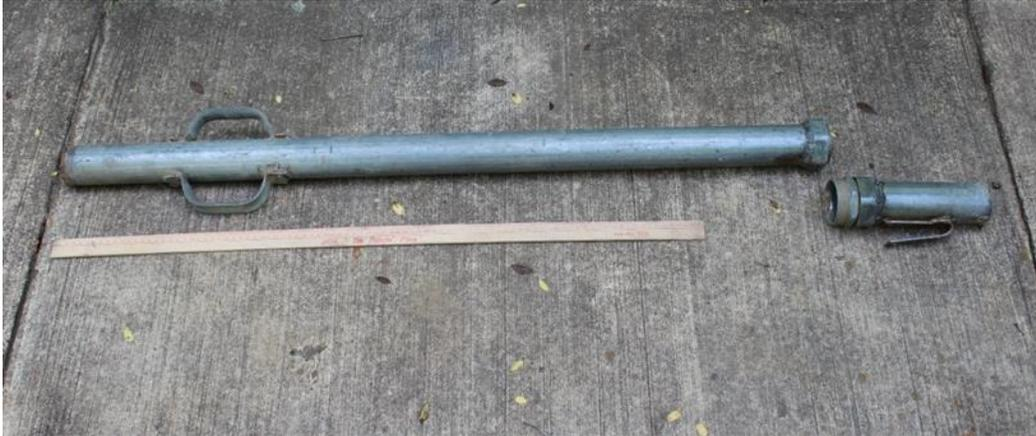
Figure 1.2 Soil-core sampling apparatus
